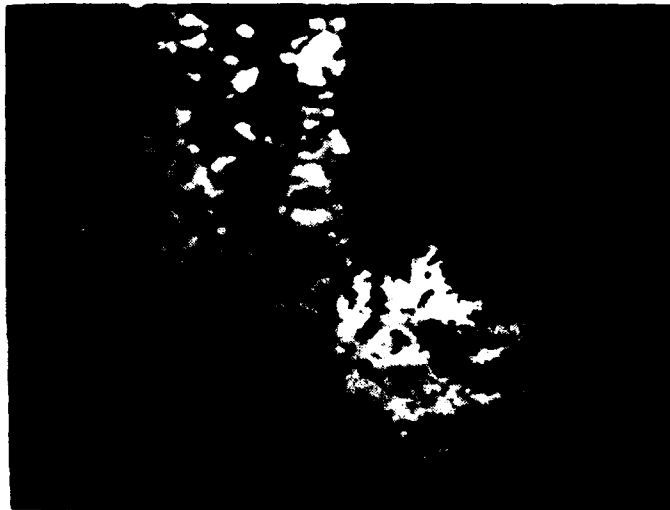
Figure 26. Lithium Dendrites on Overdischarged Cathode (3.8X Magnification); 331 Hours on Open Circuit, 2 Sec Exposure
