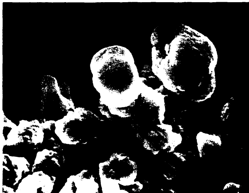
Figure 36. SEM Photograph of Lithium Dendrite Tips of Cathode Shown Above (3000X Magnification)
