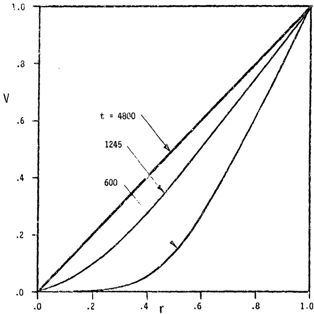
Figure 1.  $V$  vs  $r$  for Case 1 with  $c/a = 3.120$ ,  $Re = 4 \times 10^4$  at Three Values of  $t$ ;  $\tau_s = 1245$ . Laminar Ekman Layer.
