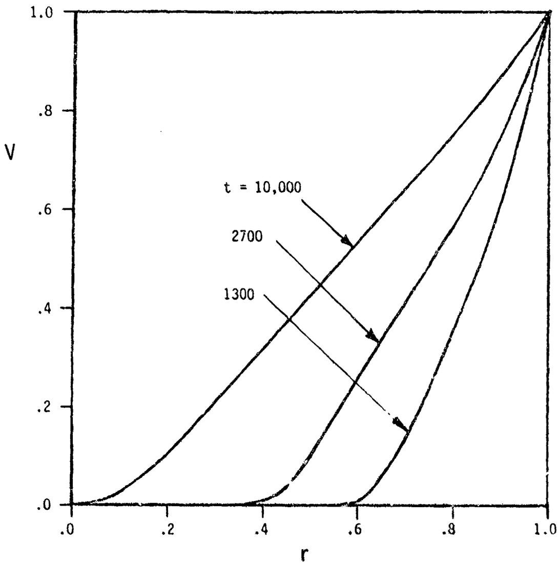
Figure 2.  $V$  vs  $r$  for Case 2 with  $c/a = 5.200$ ,  $Re = 2 \times 10^6$  at Three Values of  $t$ ;  $t_{st} = 2700$ . Turbulent Ekman Layer.
