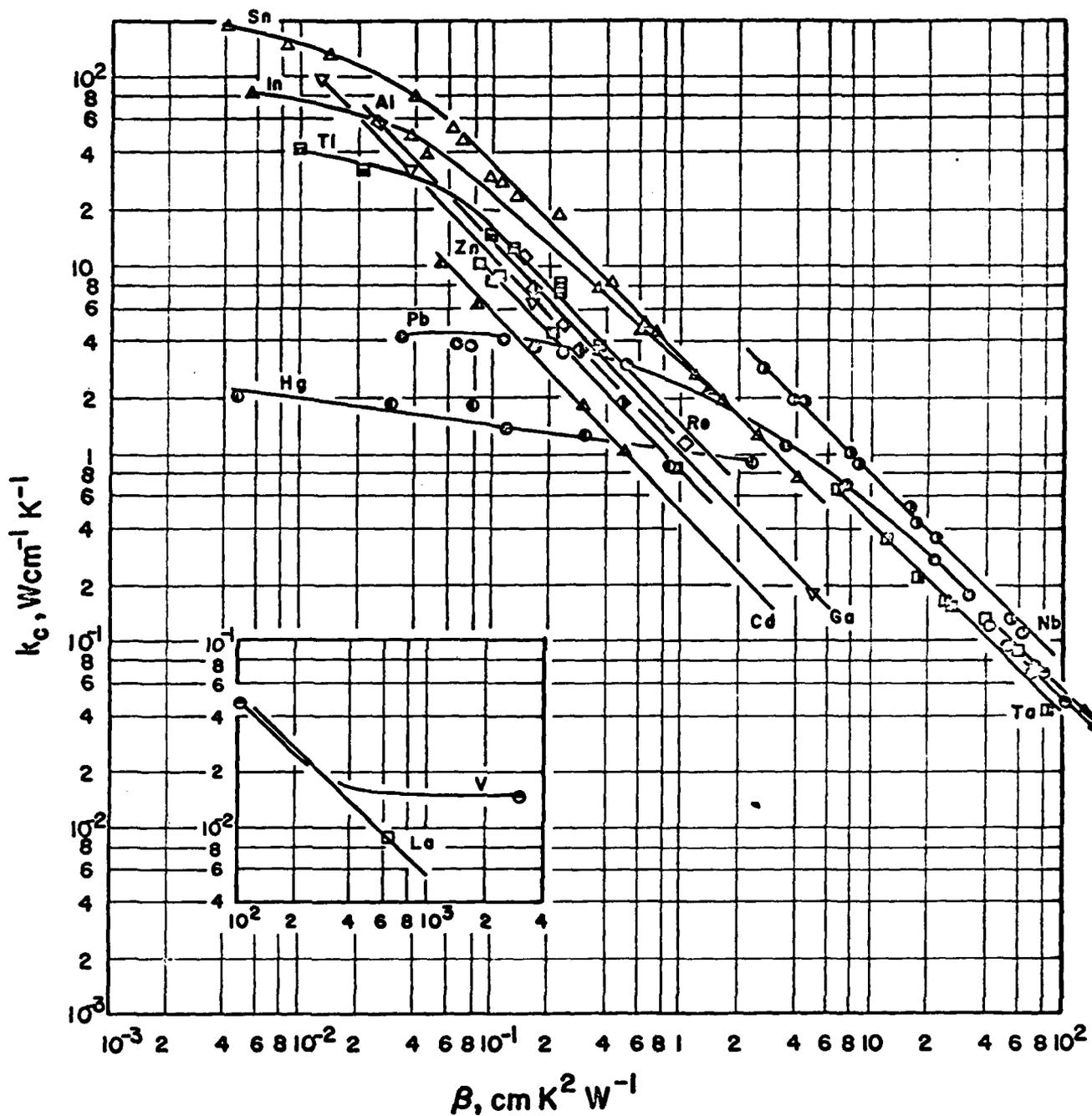
Figure 2. Thermal Conductivity at the Transition Temperature as a Function of Impurity Parameter for 14 Superconducting Elements.
