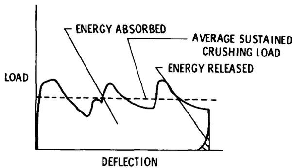
Figure 4. - Typical load-deflection curve of aluminum tube.
