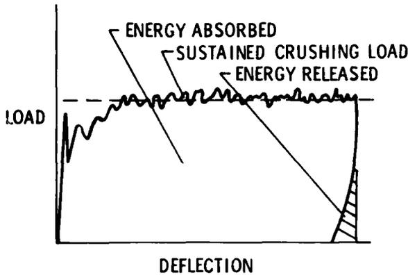
Figure 3. - Typical load-deflection curve of composite tube.
