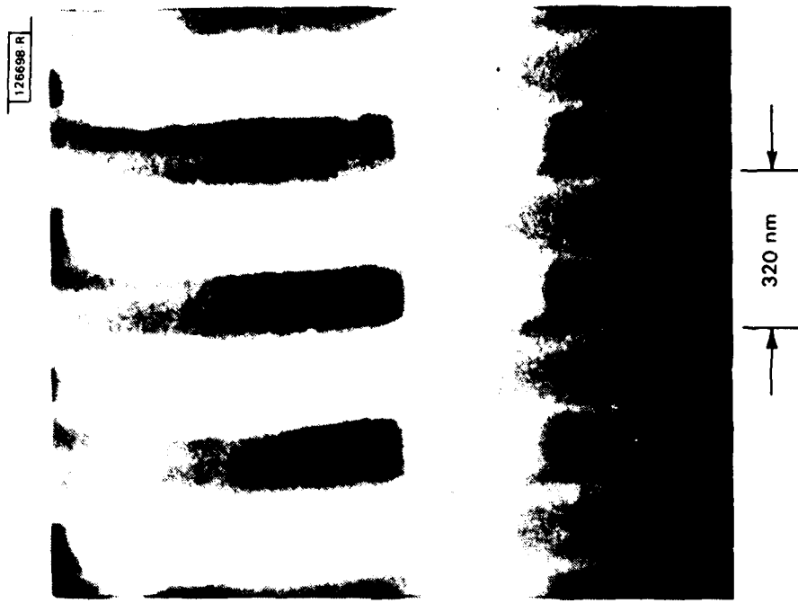
(a) (b) Fig. 4-10. SEM micrographs of 320-nm-period grating etched by RIE into ion lithography stencil mask materials: (a) a SIN structure produced by CF_4 RIE, (b) an N-O-N structure produced by CHF_3 RIE.
