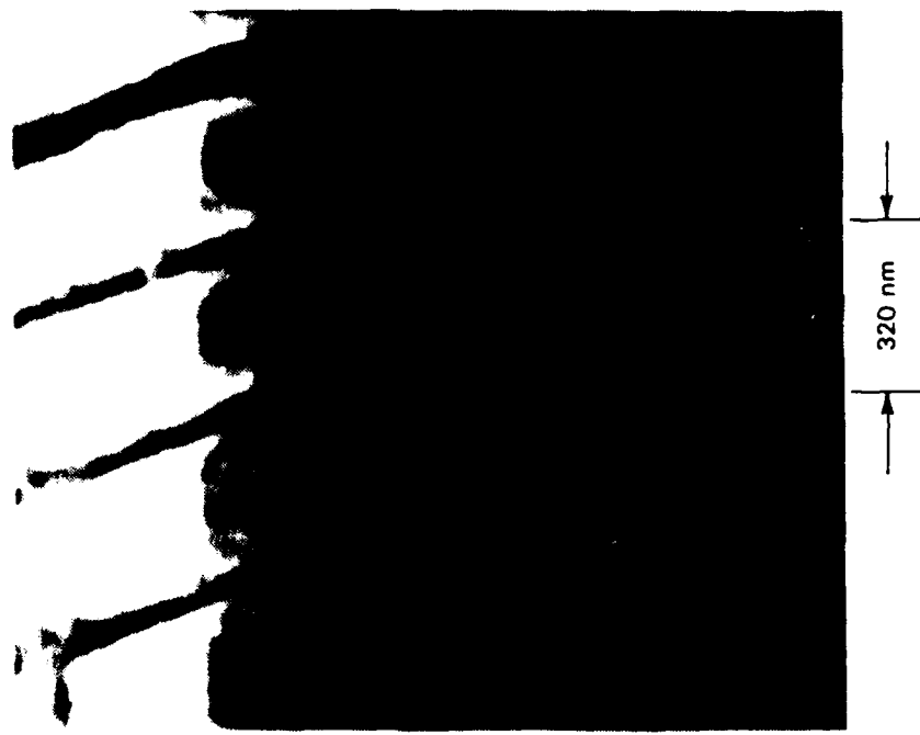
(a) (b) Fig. 4-10. SEM micrographs of 320-nm-period grating etched by RIE into ion lithography stencil mask materials: (a) a SIN structure produced by CF_4 RIE, (b) an N-O-N structure produced by CHF_3 RIE.
