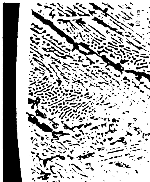
Fig. 1 - Cross section of Fe-4C sample which has been surface melted with TEA laser pulses.
