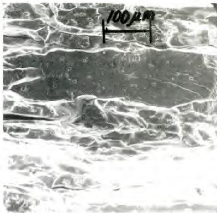
Figure 4.3e. Fracture appearance in mercury under static fatigue load control conditions for 1100-0, \Delta K \sim 8 \text{ MPa}\sqrt{\text{m}} . Crack growth in the LS plane. The fracture mode is predominantly brittle intergranular with some cleavage.
