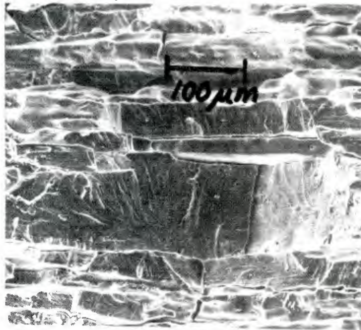
Figure 4.11d. Fracture appearance at -25°C (248°K) under static fatigue conditions for 6061-T651. K > \sim 5 \text{ MPa}\sqrt{\text{m}} . Crack growth in the LS plane, in a mixed transgranular and intergranular mode.
