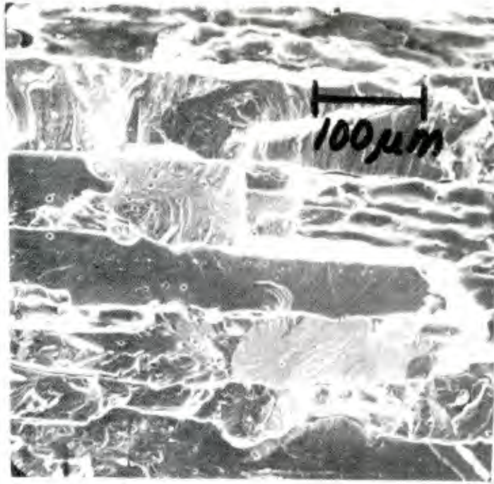
Figure 4.11c. Fracture appearance at 0°C (273°K) under static fatigue conditions for 6061-T651. K > \sim 10 \text{ MPa}\sqrt{\text{m}} . Crack growth in the LS plane, following a mixed intergranular and transgranular path.
