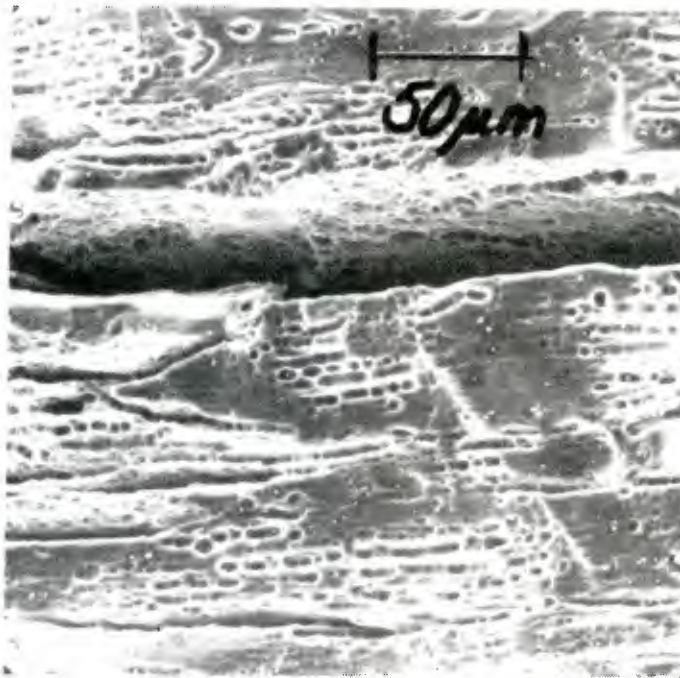
Figure 4.3d. Higher magnification of Figure 4.3c, showing dimples.
