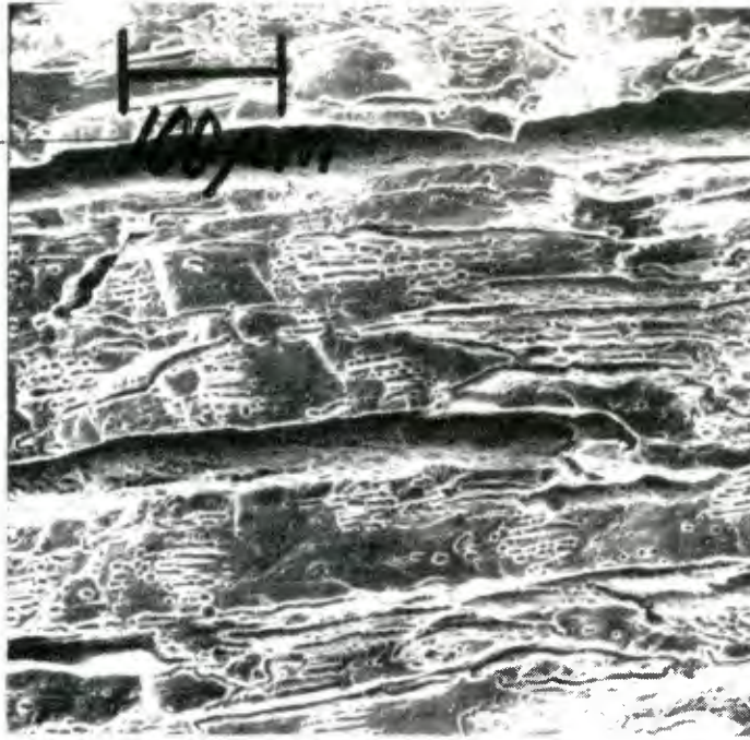
Figure 4.3c. Fracture surface in mercury for 1100-O under static fatigue, load control conditions, \Delta K > \sim 8 \text{ MPa}\sqrt{\text{m}} with either K increasing or K decreasing. Crack growth in the LS plane. The fracture mode is dimpled intergranular.
