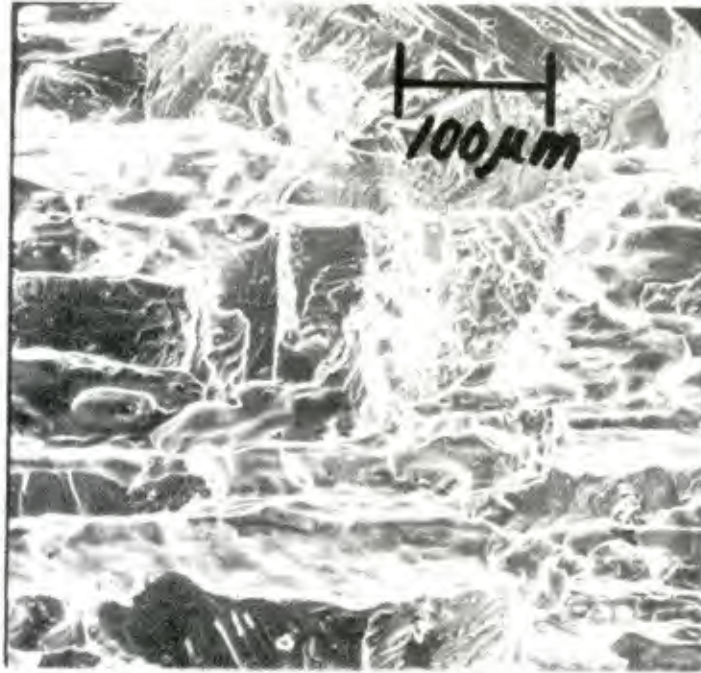
Figure 4.11a. Fracture appearance in mercury at 45°C (318°K) under static fatigue conditions for 6061-T651. K > \sim 16 \text{ MPa}\sqrt{\text{m}} . Crack growth in the LS plane, following an intergranular path.
