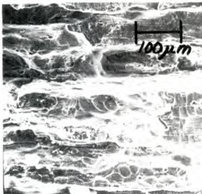
Figure 4.6c. Fracture appearance in mercury under static fatigue conditions for 6061-T651. \Delta K \sim 9 \text{ MPa}\sqrt{\text{m}} . Crack growth in the LS plane. The fracture path is intergranular.
