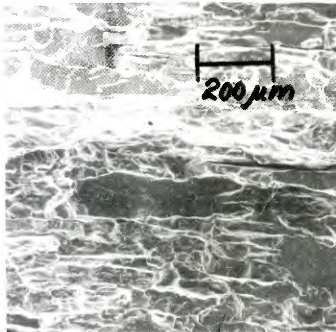
Figure 4.3f. Higher magnification of Figure 4.3e showing the apparently cleaved grain and small dimples.
