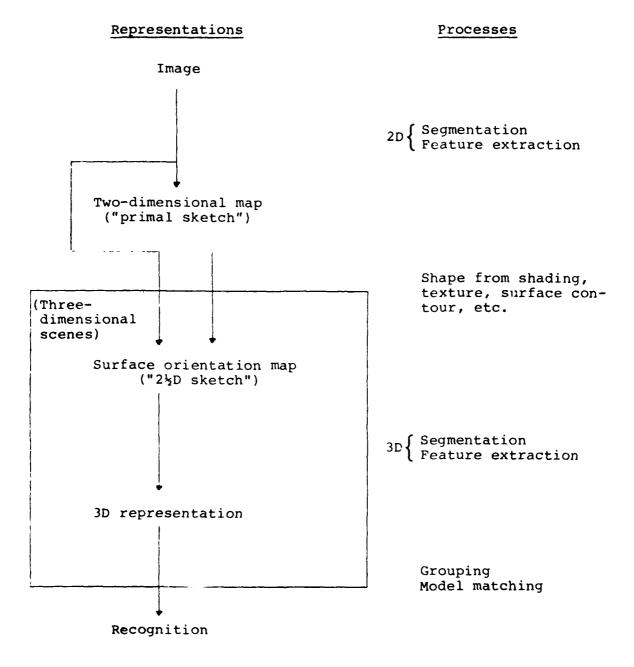
Figure 1. Simplified diagram of a computer vision system.
