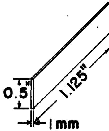
Figure 7. Propellant Slabs
