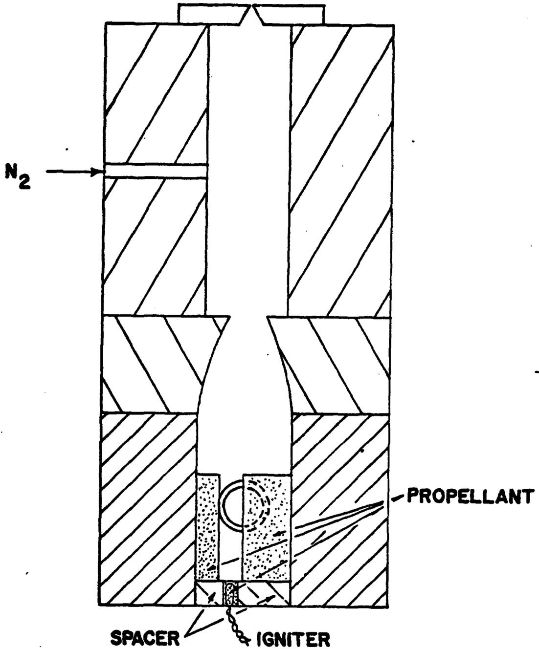
Figure 6. Motor Line Drawing, Window Side View
