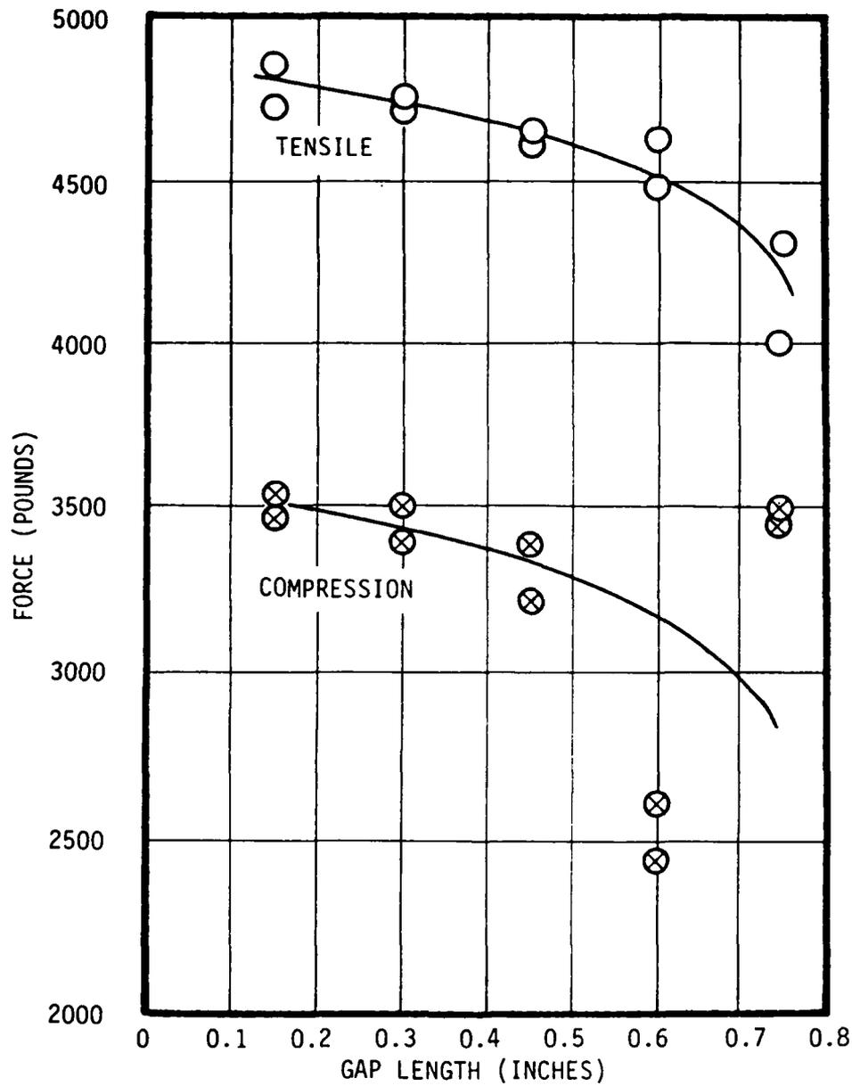
Figure 13. Compressive and tensile forces for 3/4-inch control tube coupling versus end gap spacing.
