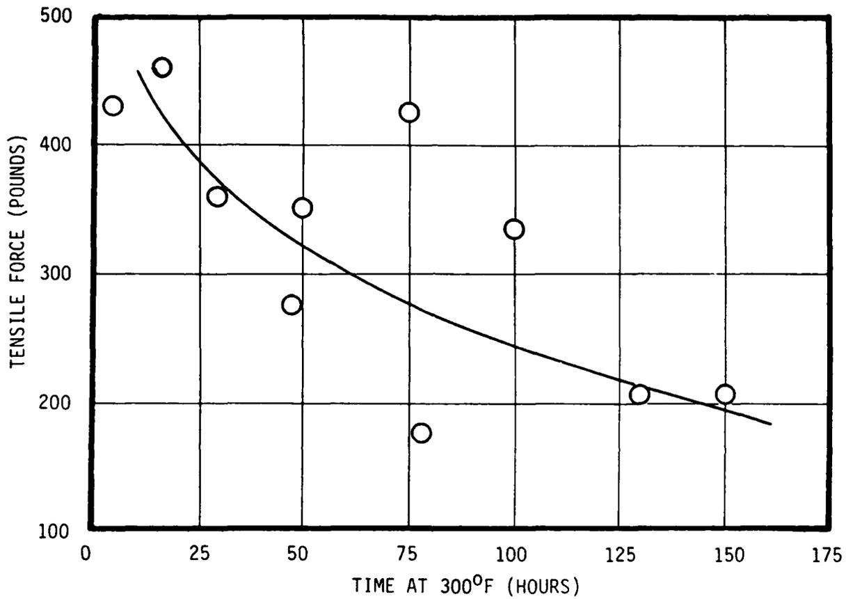
Figure 15. Tensile performance of a 3/4-inch split-ring coupling versus time soaked at 300°F.
