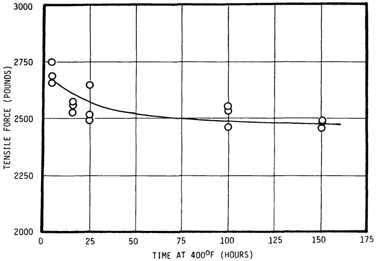
Figure 12. Tensile force for 3/4-inch control tube coupling versus temperature soak; annealed liners; minimum gap spacing.
