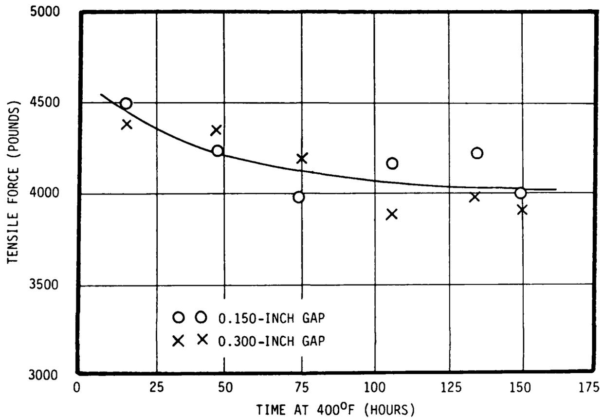
Figure 11. Tensile force for 3/4-inch control tube couplings versus temperature soak, unannealed liners.
