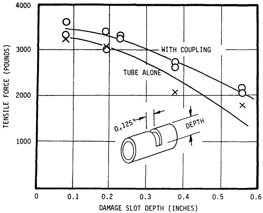
Figure 14. Tensile performance of 3/4-inch control tube coupling (split-ring design) versus tubing damage.
