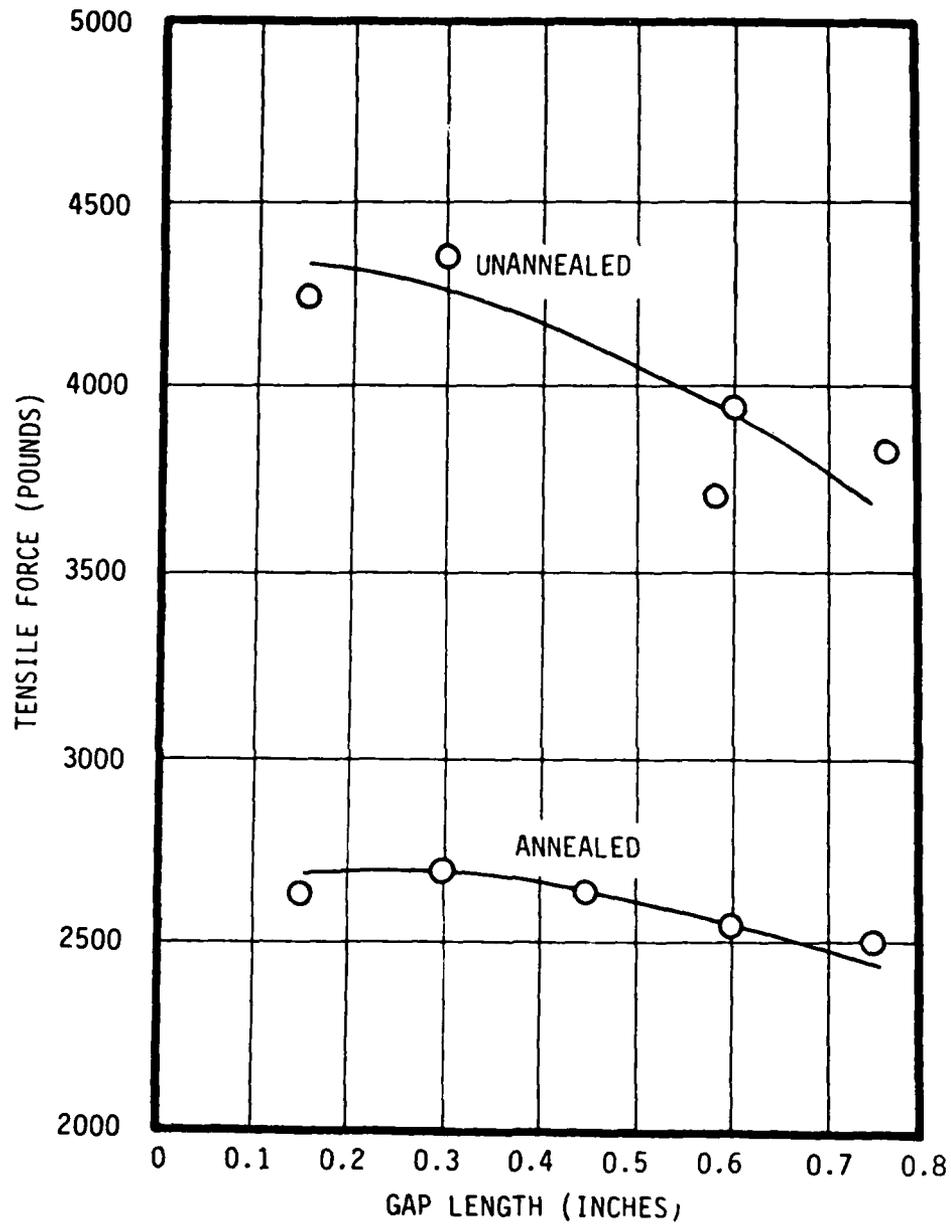
Figure 10. Tensile force for 3/4-inch couplings versus end gap spacing.
