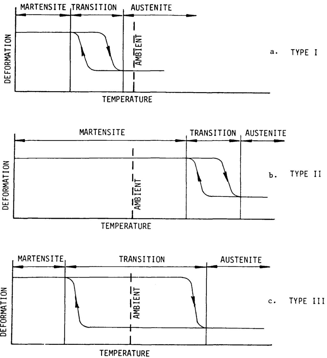
Figure 2. Illustration of shape memory alloy types and transformation temperatures.
