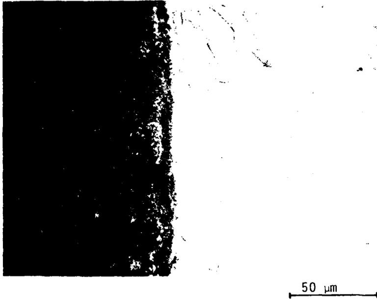
FIGURE 37. DETAIL OF FIGURE 35. THE 1010 INTERLEAF IS AT THE RIGHT. MAGNIFICATION: 500X. 2% NITAL ETCHANT.
