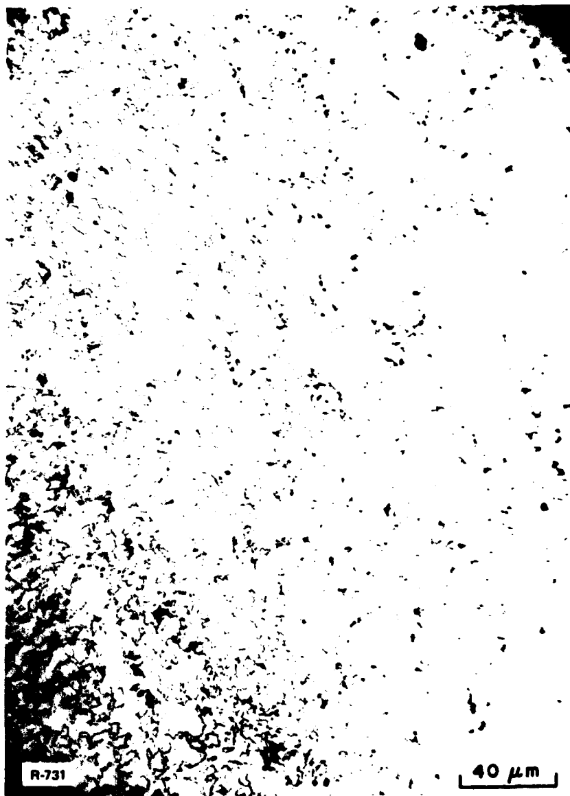
Figure 1 - Microstructure of MF-80 HSLA steel viewed in short transverse direction
