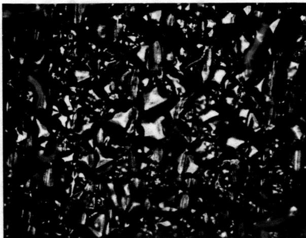
FIGURE 2-12. (111) TEXTURED CdTe ON SAPPHIRE GROWN AT
