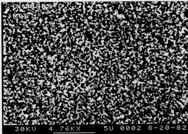
FIGURE 3-5(a). SEM MICROGRAPH OF CdTe FILM DEPOSITED ON SAPPHIRE BY HWE, 2 MICRONS THICK.
