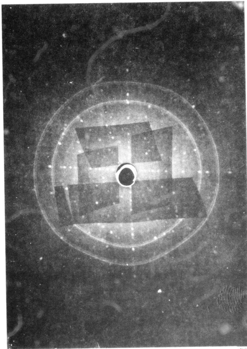
FIGURE 2-21. BACK REFLECTION LAUE X-RAY DIFFRACTION PATTERN FROM POLYCRYSTALLINE  $\text{HgCdTe}$  FILM ON A SINGLE CRYSTAL SAPPHIRE SUBSTRATE
