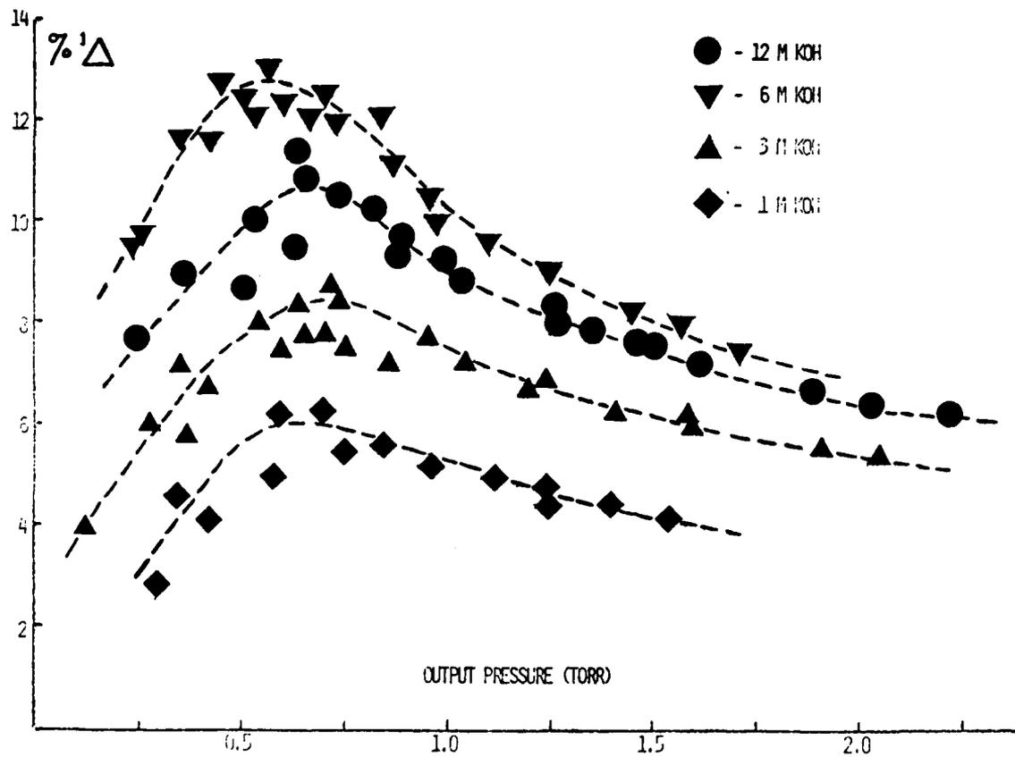
Fig 4. Effect of initial KOH molarity on  $O_2(^1\Delta)$  %.
