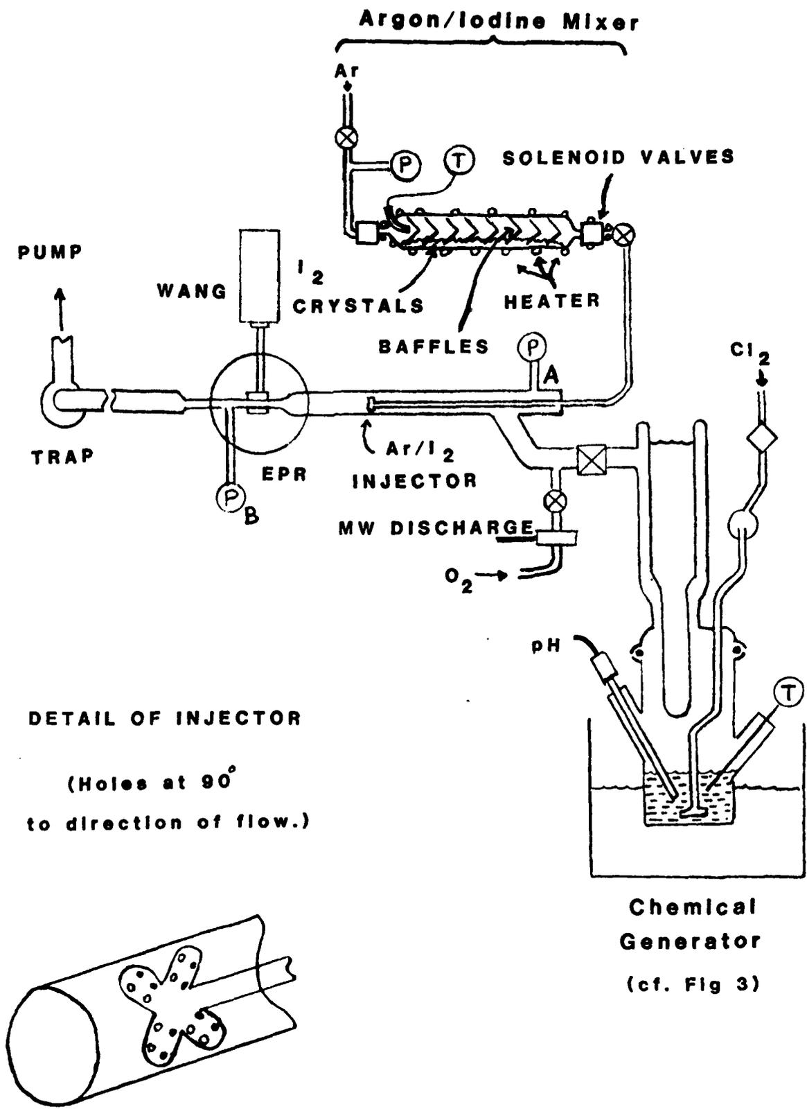
Fig 7. Flow system for EPR studies
