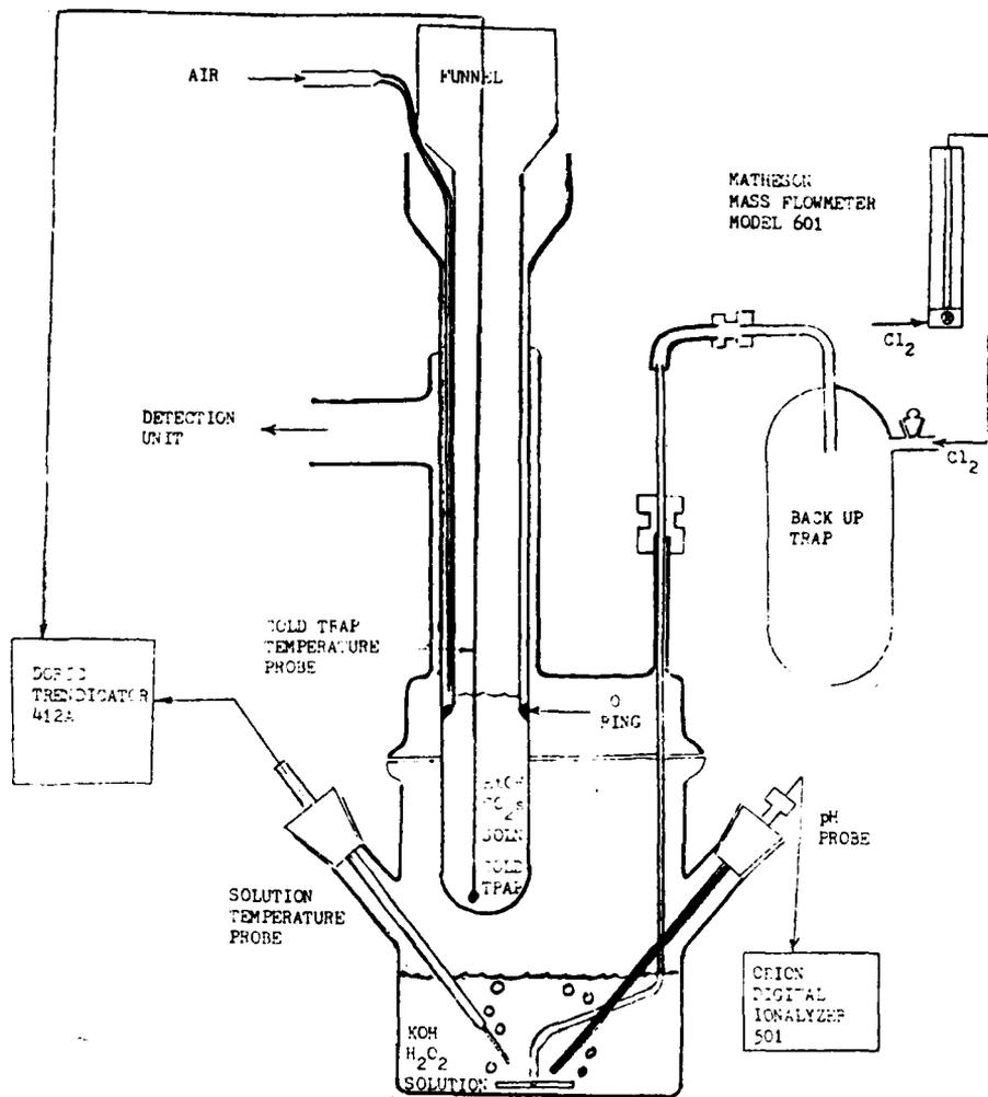
Fig 3. Small-scale generator with variable trapping surface.
