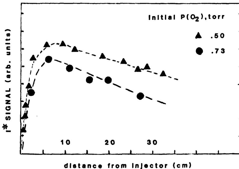
Fig 9.  $I^*$  signal in EPR cavity as a function of distance from injector in flow tube.  $O_2$  flow at 20 SCCS.
