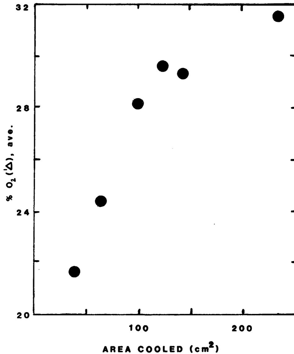
Fig 6. Plot of % O<sub>2</sub>(<sup>1</sup>Δ) average (for readings in first 10 minutes of each run) vs. area of in-reactor trap surface cooled to -78°C.
