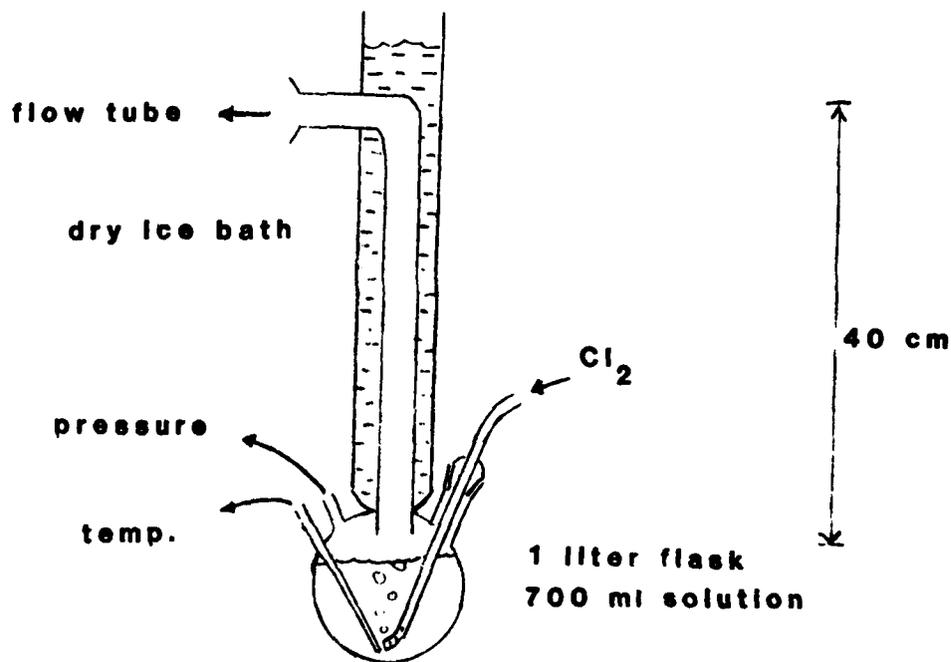
Fig 8. Batch reactor with flow-through trap configuration.
