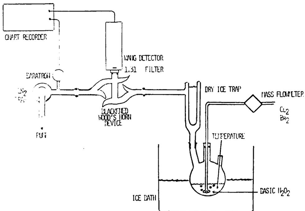
Fig 1. Small scale batch reactor flow apparatus.
