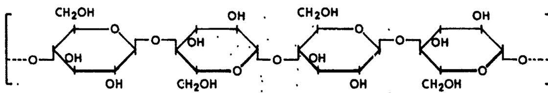
Figure 1. Cellulose [ $\beta(1,4)$  D-Glucosepyranose] Molecule
