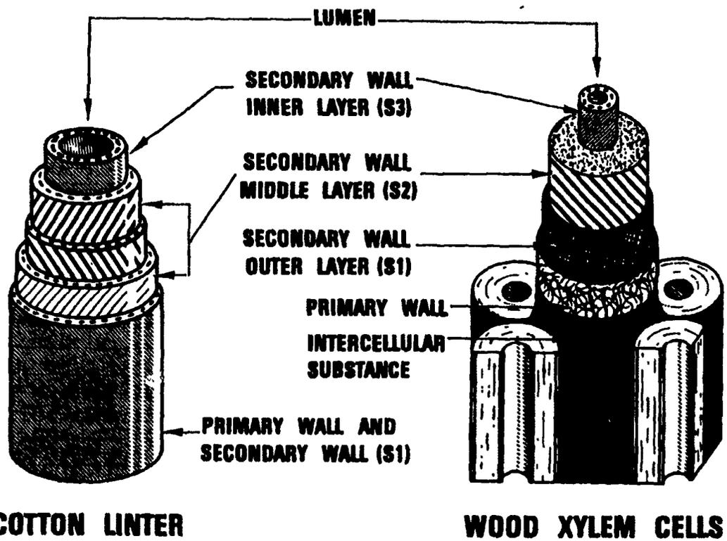
Figure 4. Model of Basic Cell Wall Structures of Cotton and Wood Cells Showing Laminar Structure of Cell Walls
