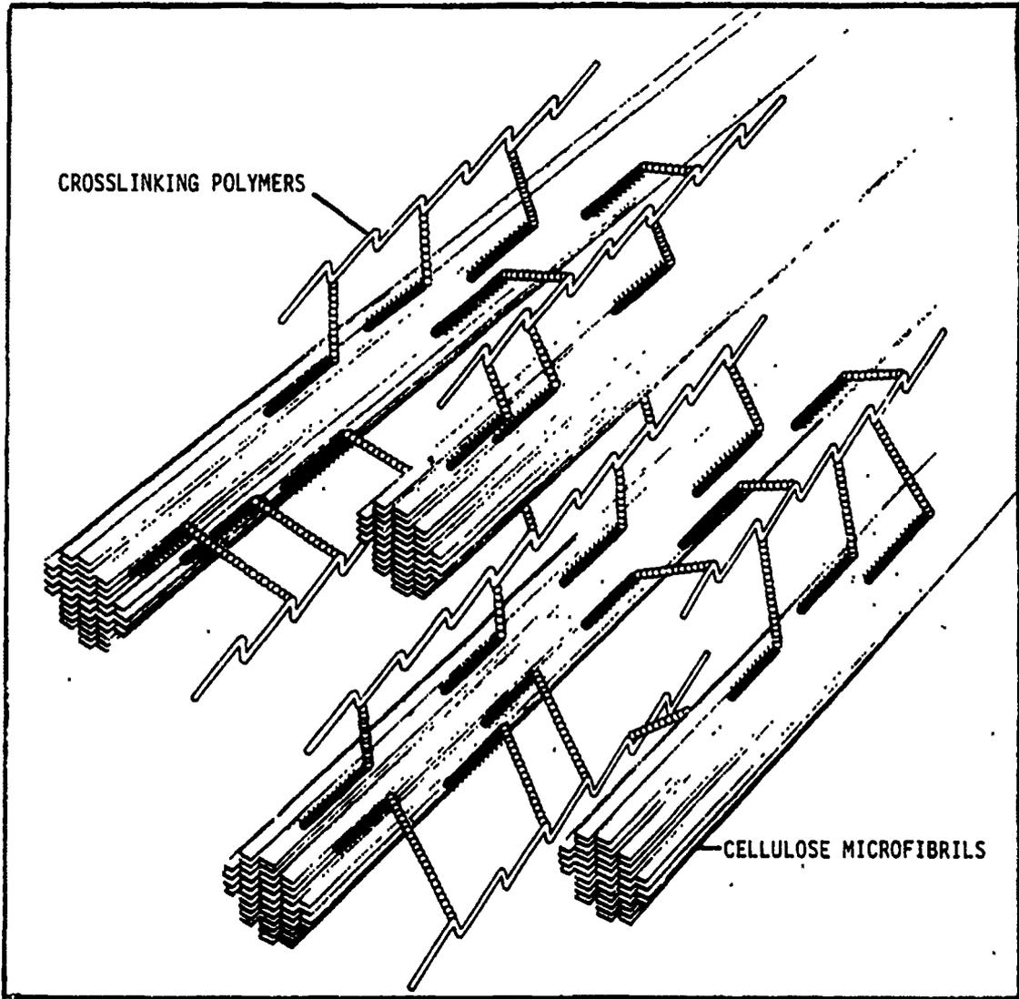
Figure 3. Model of Plant Cell Wall Bonding of Microfibril Bundles
