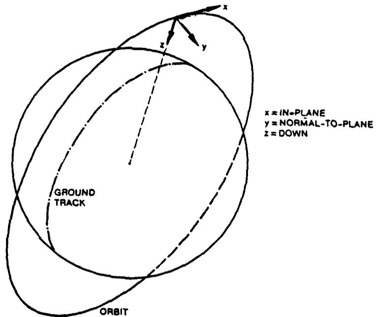
Fig. 2 - Satellite centered cartesian coordinate system
