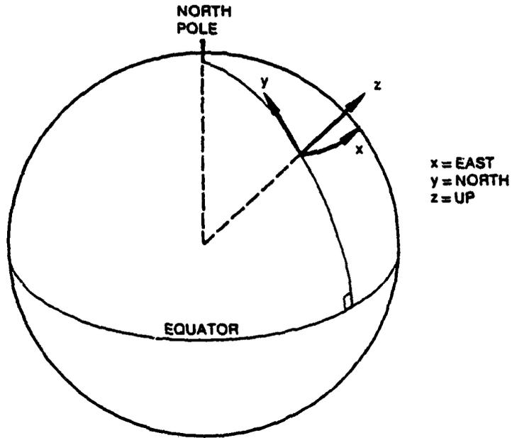
Fig. 3 — Target centered cartesian coordinate system
