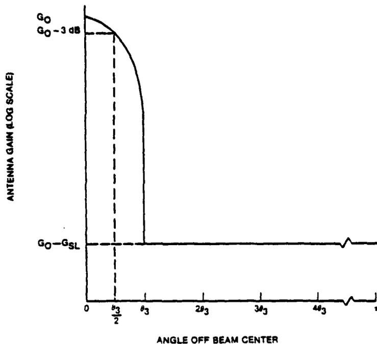
Fig. 8 - One-dimensional antenna pattern as modelled by SRM
