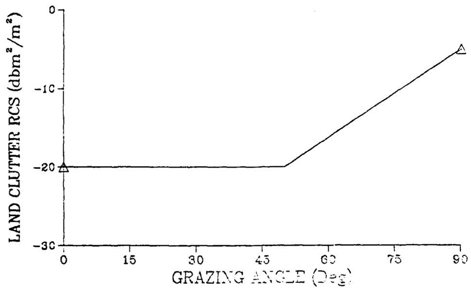
Fig. 11 - Space Radar Model land clutter RCS model
