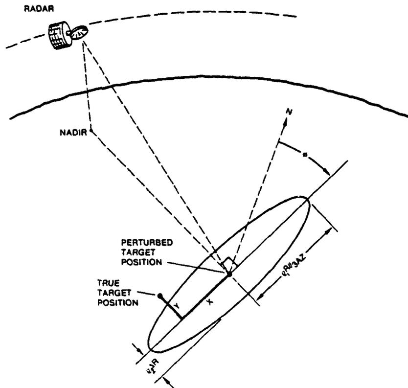
Fig. 12 — Detection error ellipse geometry showing semi-major and semi-minor axis lengths and ellipse orientation
