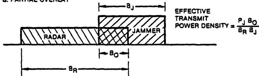
Fig. 9 - Illustration of jammer effective transmit power density for cases of full and partial overlap of jammer bandwidth where  $B_O = B_R - B_J$
