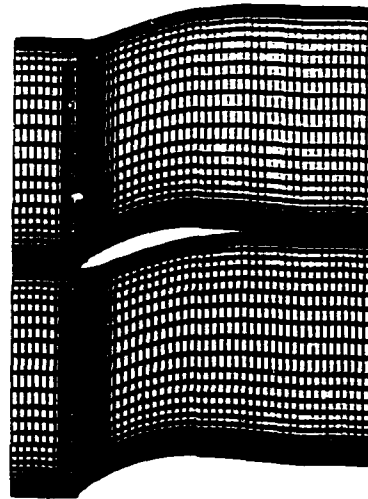
Figure 11. 73x34 grid for supercritical stator
