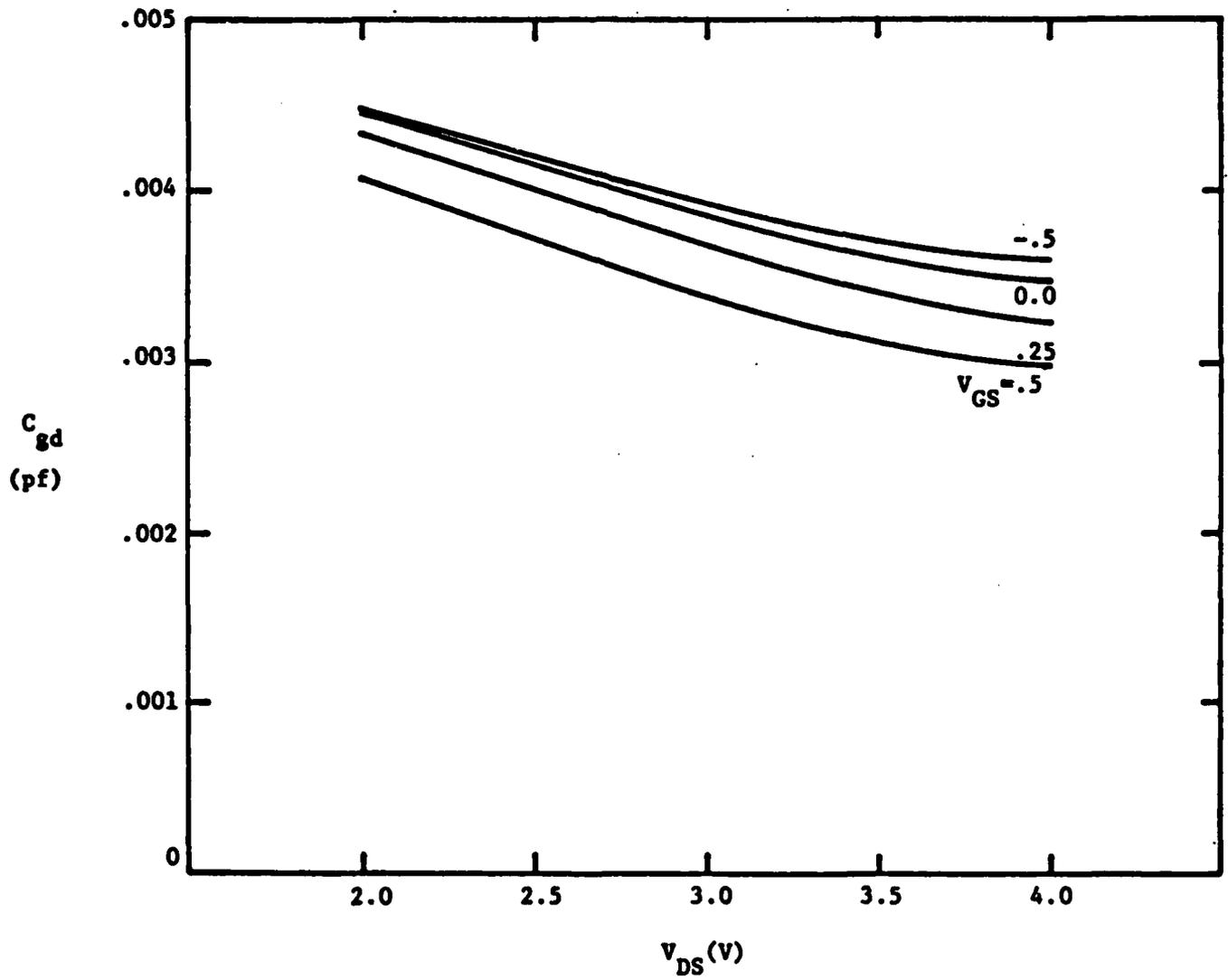
Fig. 19  $C_{gd}$  for ion-implanted FET.
