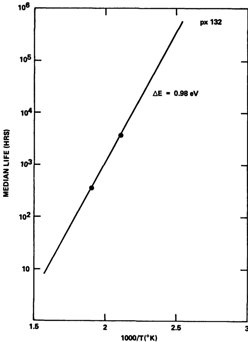
Fig. 9 Arrhenius plot for the median lifetime of 9-stage ring oscillators. Failure was defined as the point when the oscillation frequency at the given temperature degrades by 20%.
