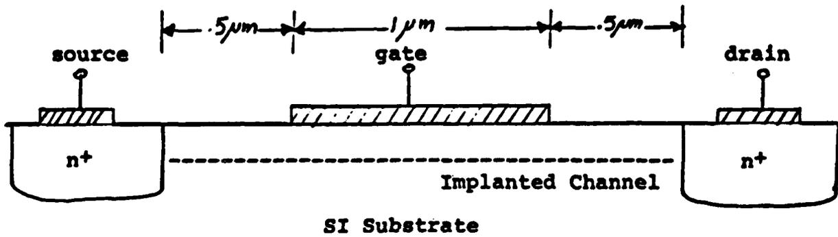
Fig. 10 FET structure used for two-dimensional analysis.
