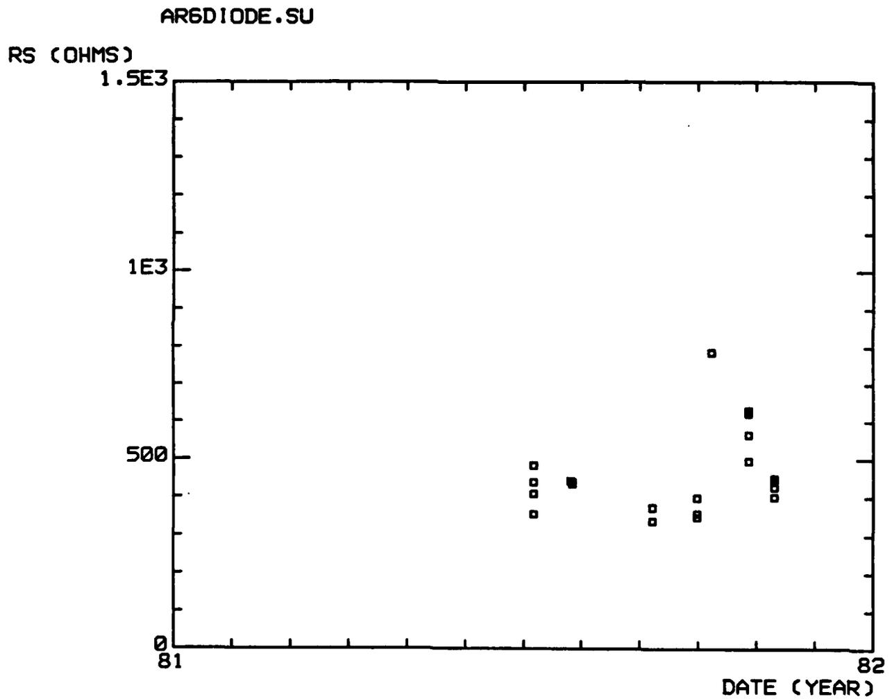
Fig.6 History of logic diode series resistance,  $R_s$ , for the AR6 wafers. Each data point represents the average over one wafer.
