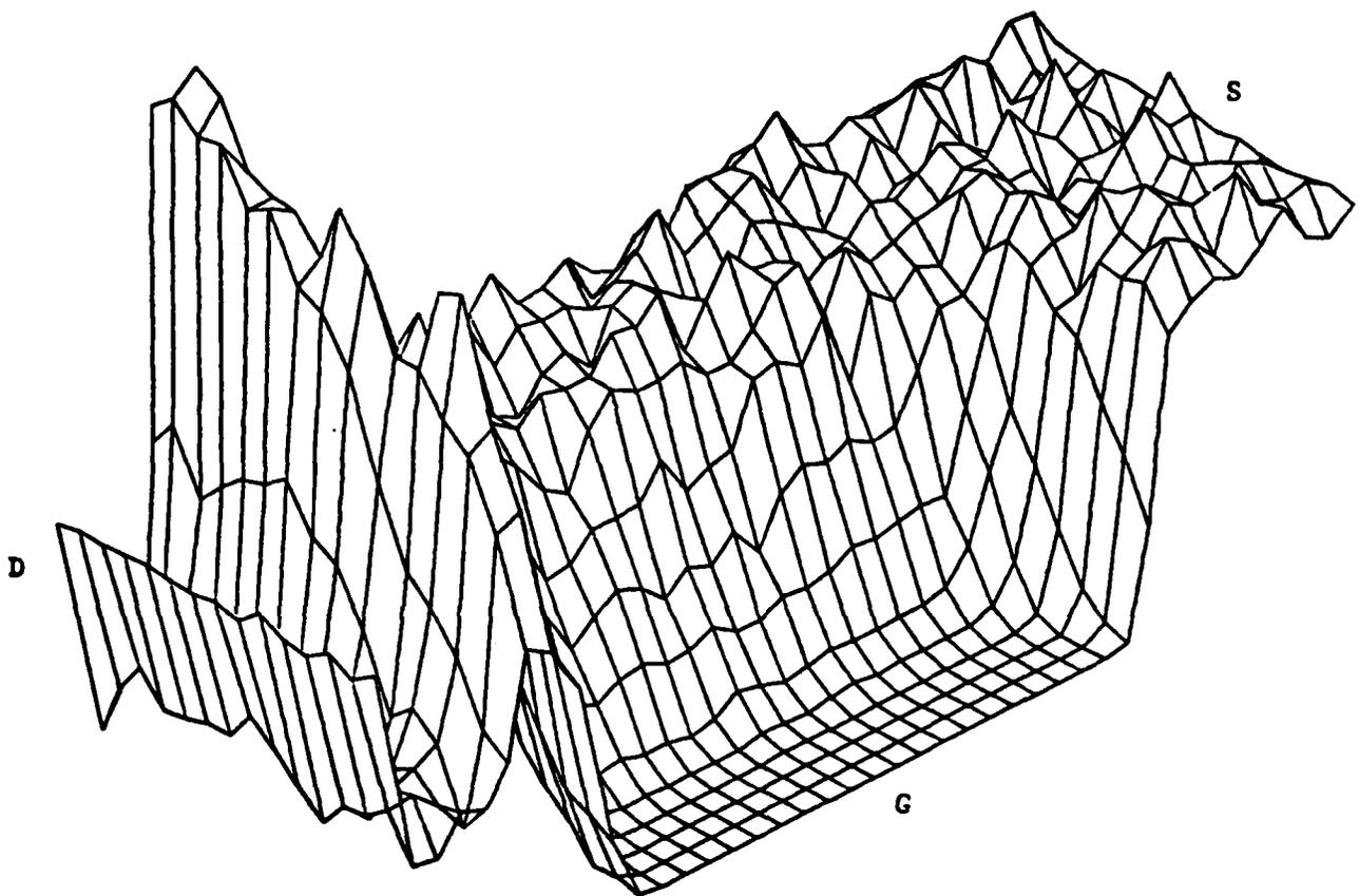
Fig. 22 Net charge density obtained a self consistent solution is reached.
