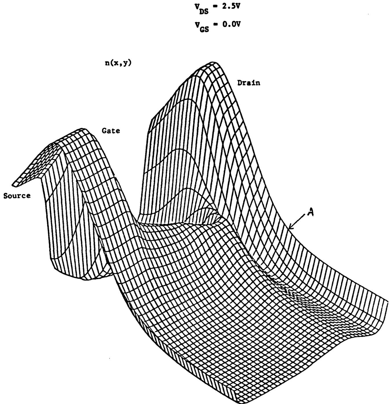
Fig. 13 Electron concentration in the channel region.
