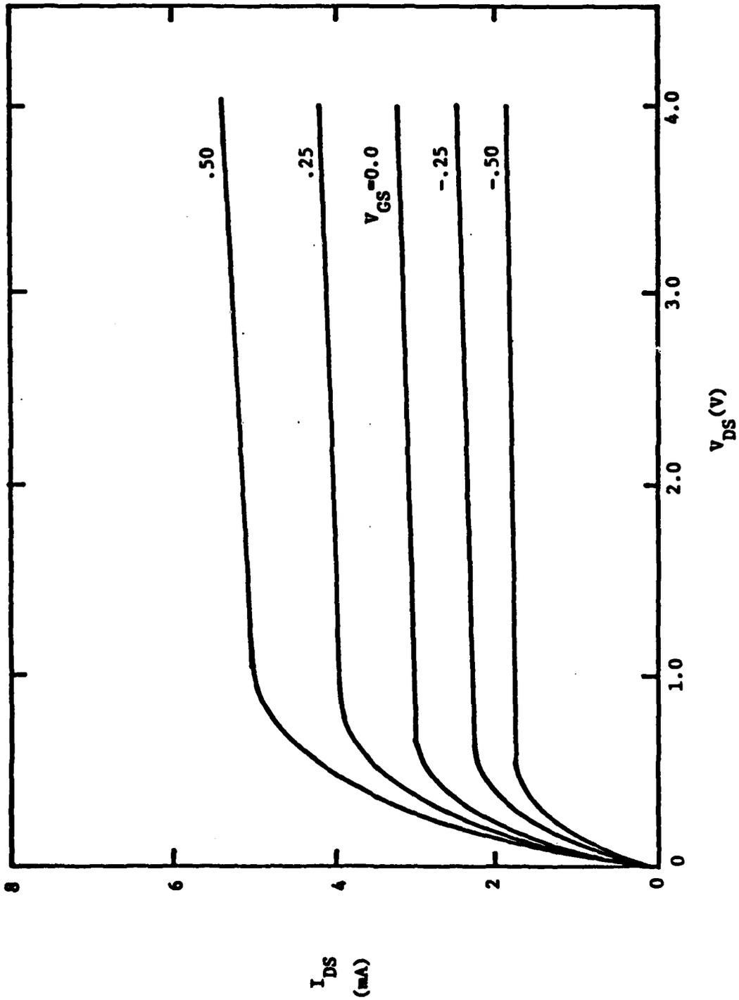
Fig. 15  $I_{ds}$ - $V_{ds}$  characteristics for ion-implanted FET.
