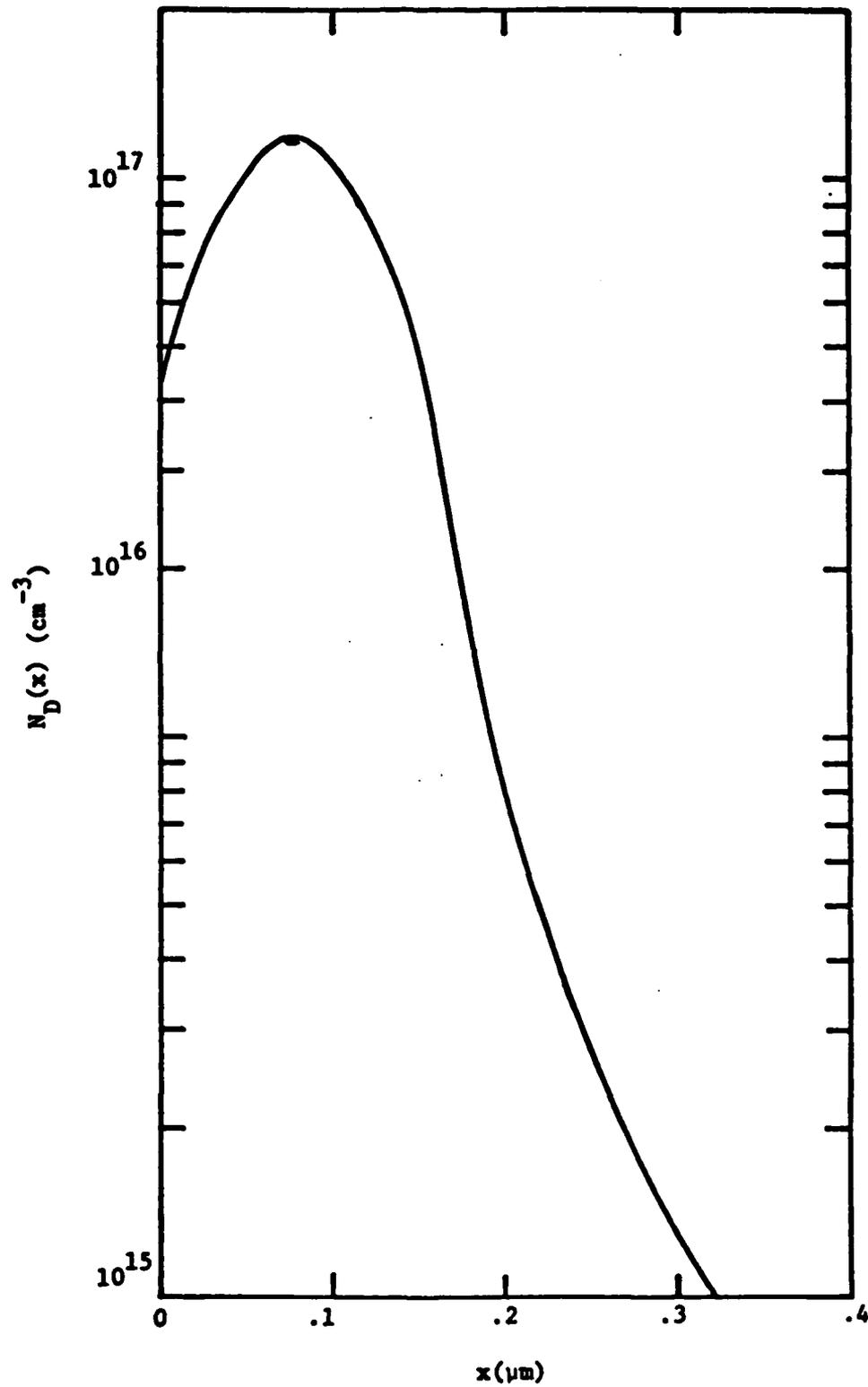
Fig. 11 Ion-implanted doping profile used in 2D modeling.
