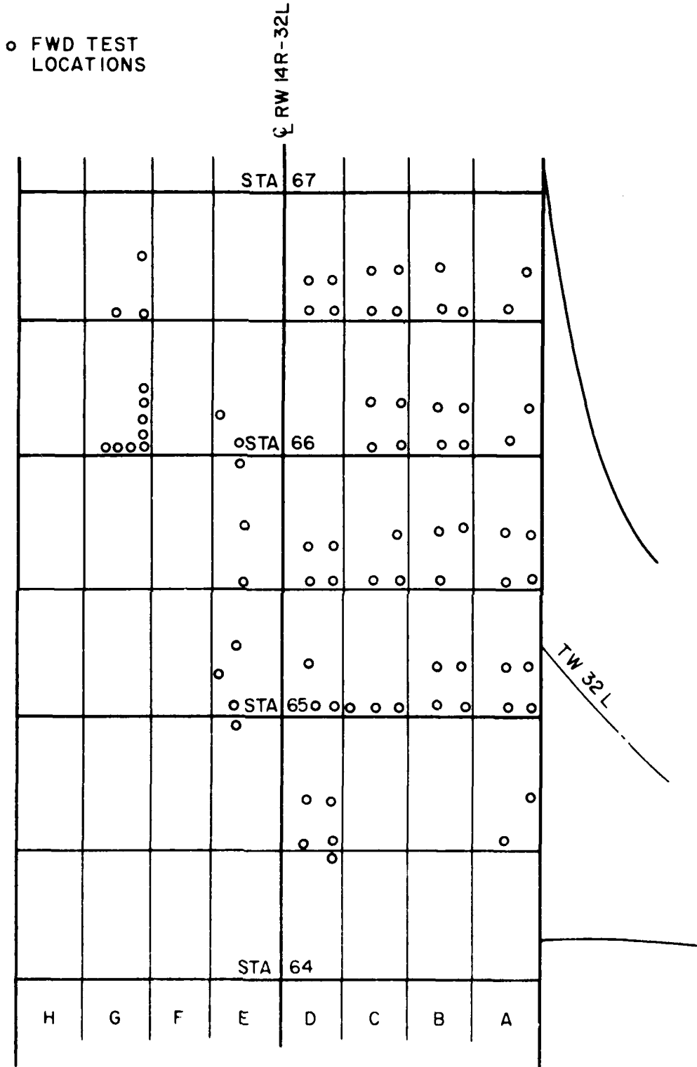
Figure 8. Locations of FWD Tests on RW 14R-32L
