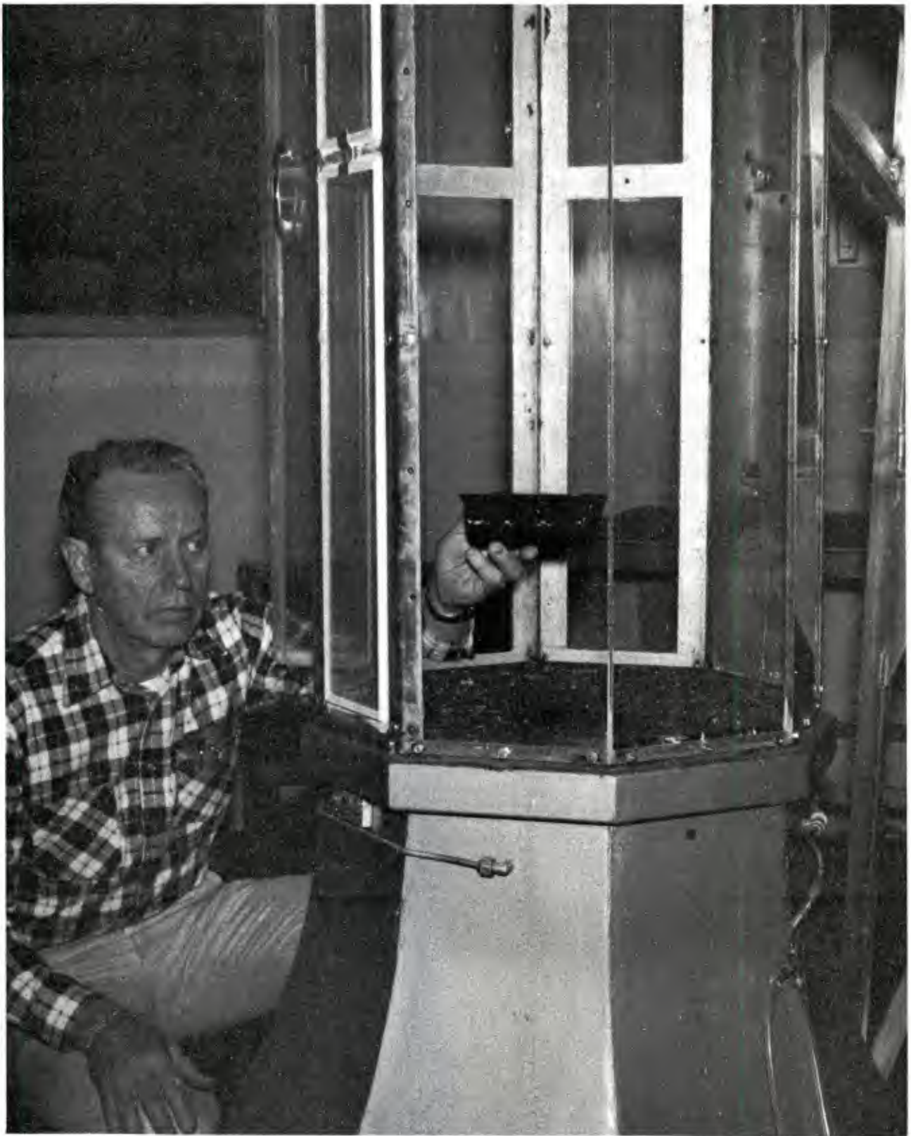
Figure 10. Typical Model Installation in 18 x 18 Inch Test Section of Vertical Wind Tunnel
