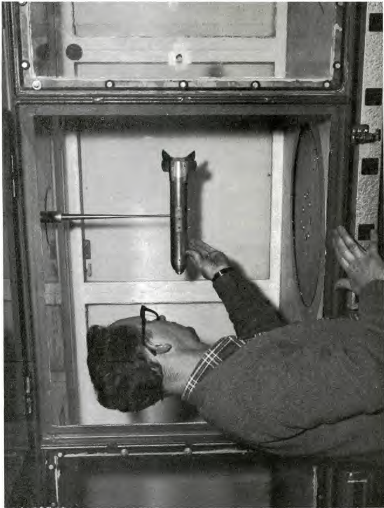
Figure 4. Typical Model Installation in 40x28 Inch Subsonic Wind Tunnel
