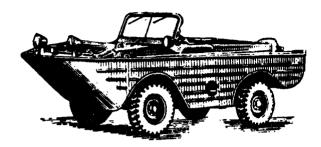
Fig. 6. Small amphibious automobile MAV.
