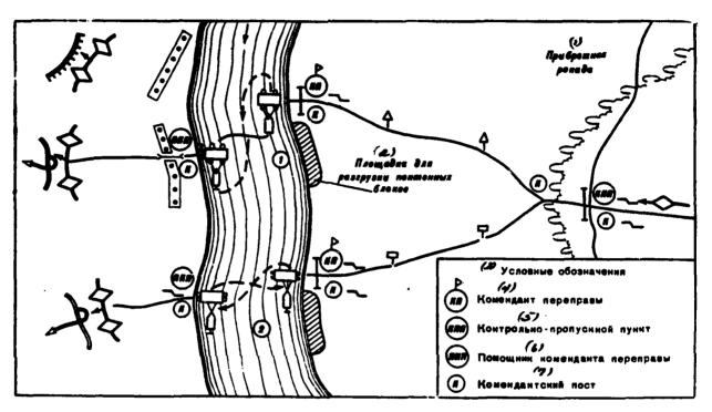
Fig. 27. Engineering armament of ferry crossings (versions): 1 - from motor pool TPP; 2 - from motor pool PMP.
