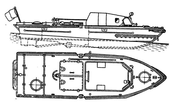
Fig. 14. Towing launch BMK-150.
