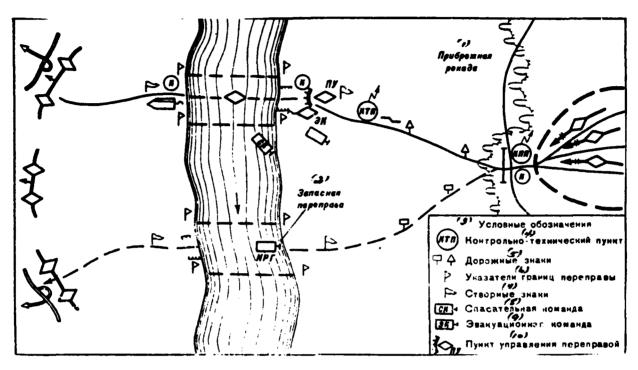
Fig. 28. Engineering armament of crossing of tanks on deep fords and under water (version).
