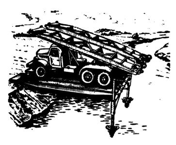
Fig. 16. Bridge layer KMM at moment of its installation/setting up to obstacle.
