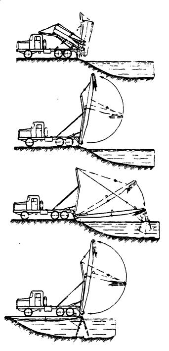
Fig. 18. Assembly diagram of bridge from set TMM.
