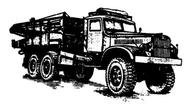
Fig. 17. Bridge layer TMM in transport position/situation.
