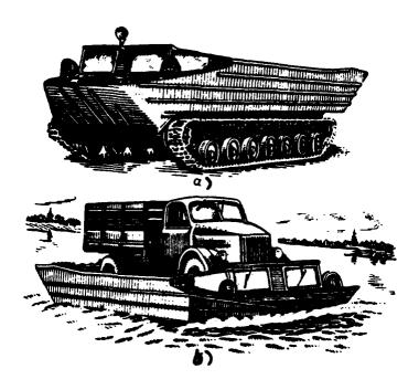
Fig. 8. Tracked amphibious personnel carrier K-61: a) on dry land; b) on the water.
