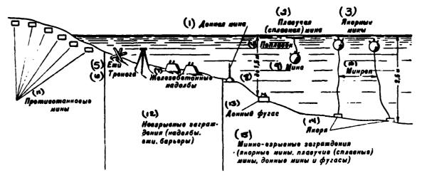
Fig. 5. Installation/setting up of engineering obstacles in the river and on the coasts.
