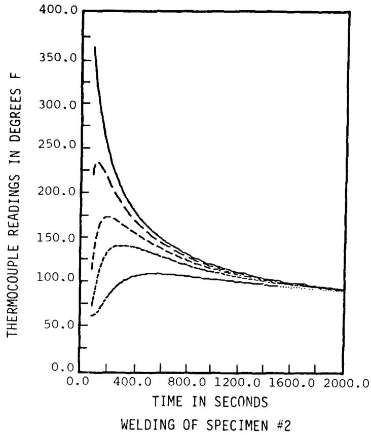
FIGURE 3.18 Thermocouple readings during welding of specimen #2
