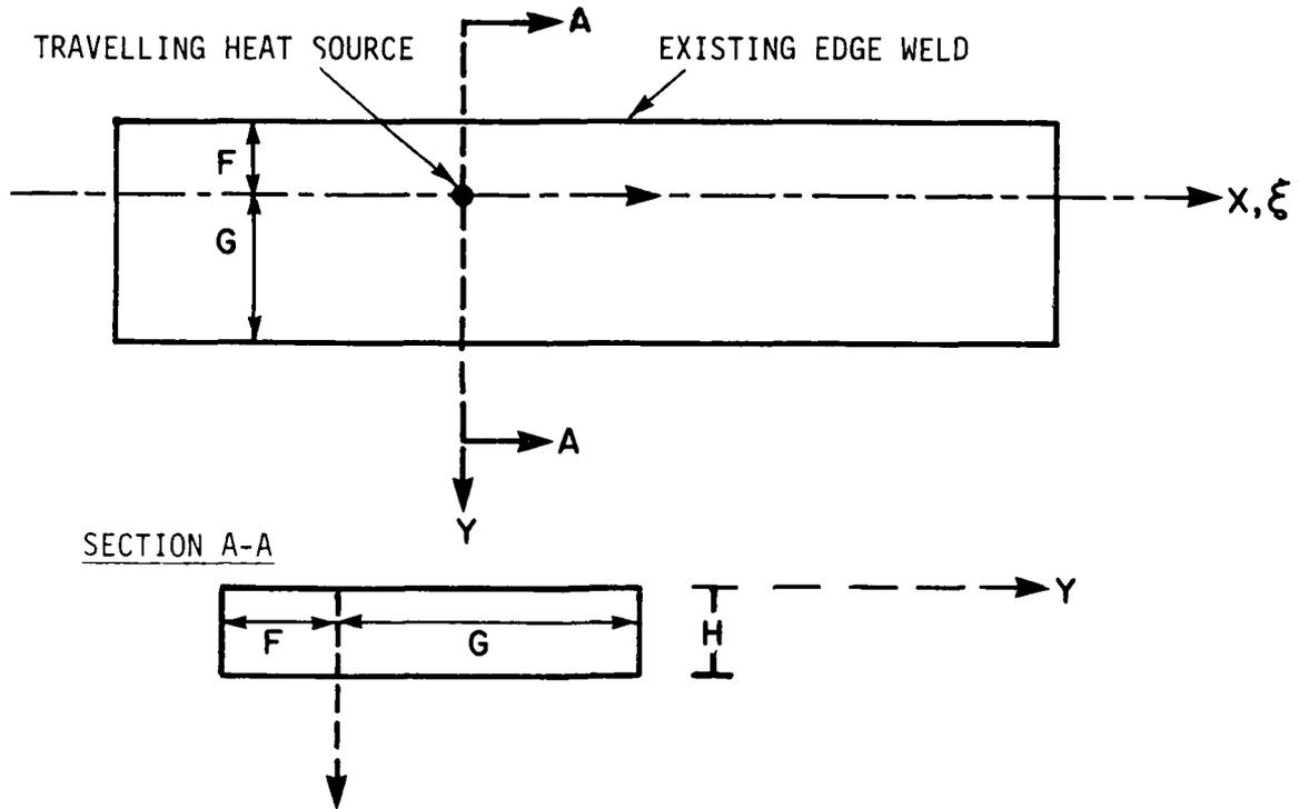
FIGURE 3.4 Geometry of plate undergoing strip heating
