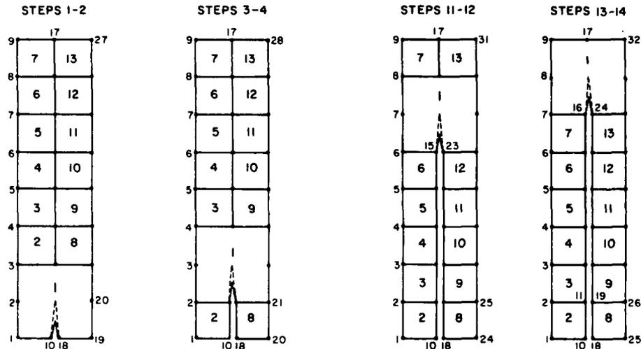
Fig. 22 Schematic representation of crack growth process
