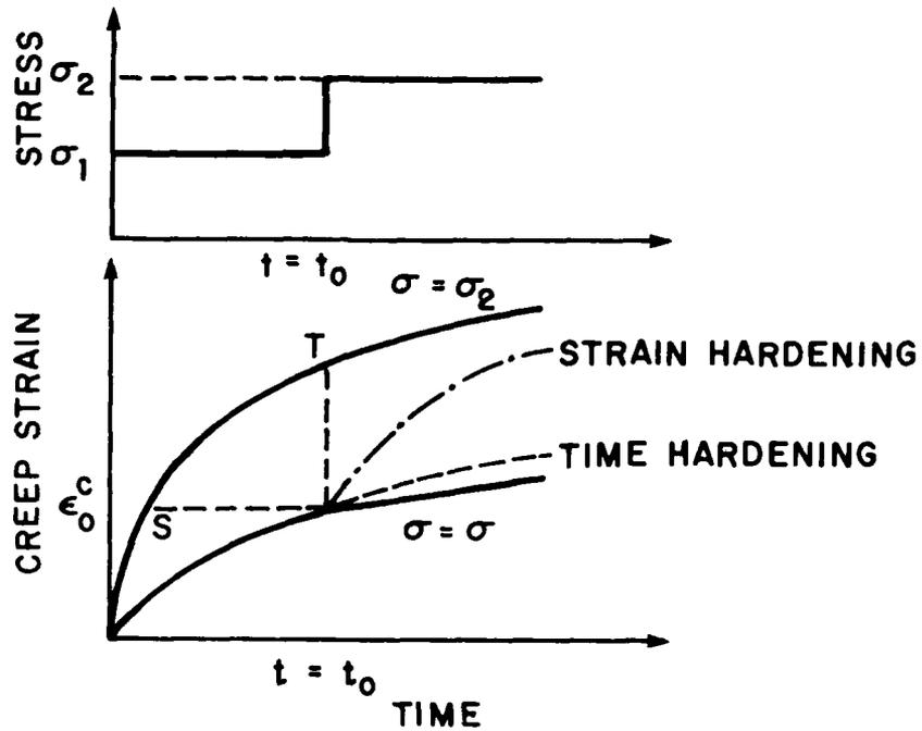
FIGURE 3.9 Strain-hardening and time-hardening models of creep response under a stepwise varying load
