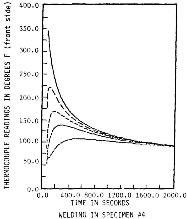
FIGURE 3.20 Thermocouple readings during welding of specimen #4
