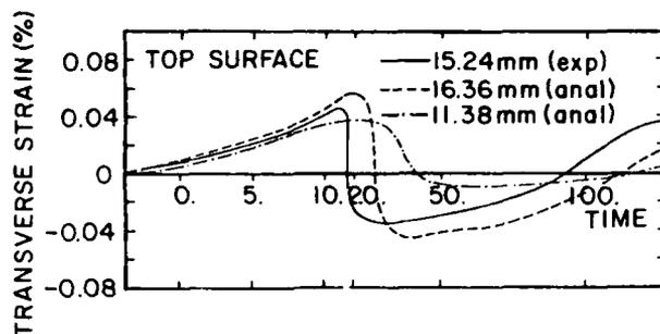
Fig. 10 Comparison of experimentally measured transverse transient strains on the plate's top surface with numerical predictions
