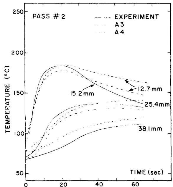
Fig. 7 Comparison of finite element results with experimental data (pass No. 2)
