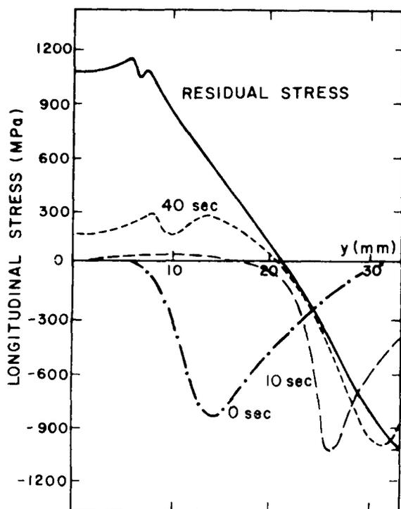
Fig. 9 Longitudinal stress distribution at several time instances
