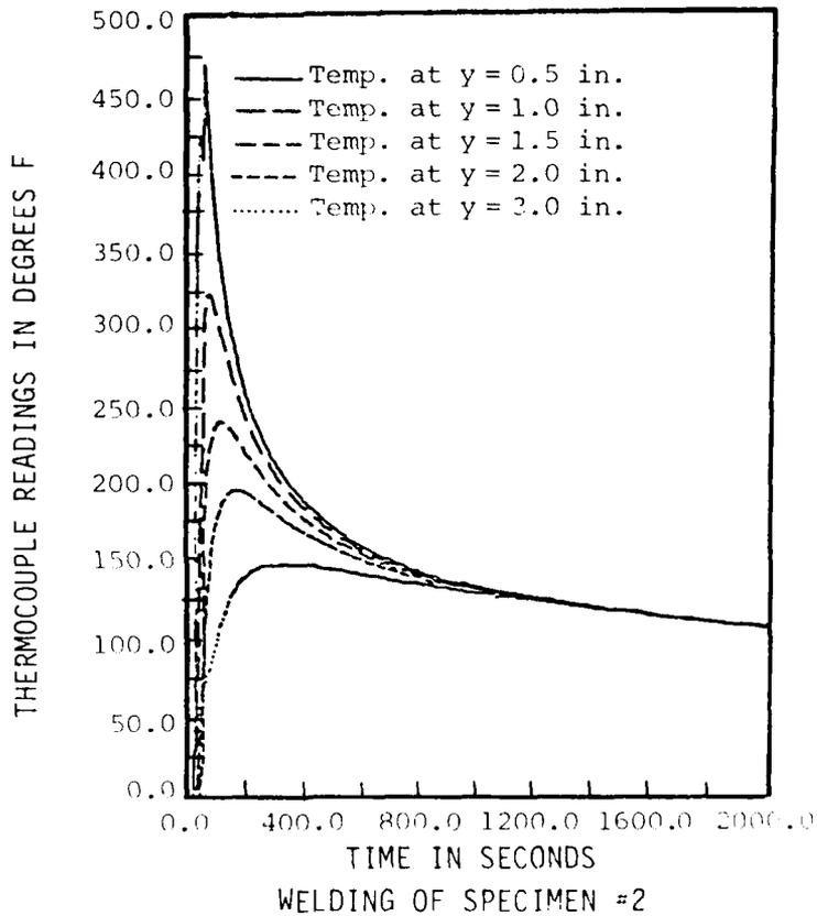
FIGURE 3.27 Time variation of temperature during welding
