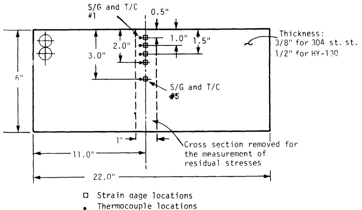
FIGURE 3.17 Specimen geometry and instrumentation
