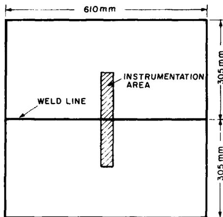
Fig. 9 Test plate arrangement
