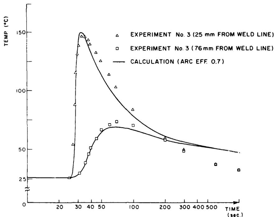
Fig. 6 Temperature distribution—analysis versus experiment (bead-on-plate weld; line heat source)
