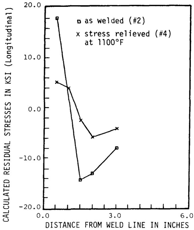
FIGURE 3.26 Comparison of longitudinal residual stresses after welding and stress relieving (1100°F)
