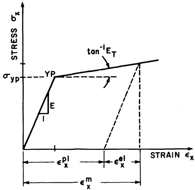
FIGURE 3.7 Bilinear stress strain law used in 1-D model
