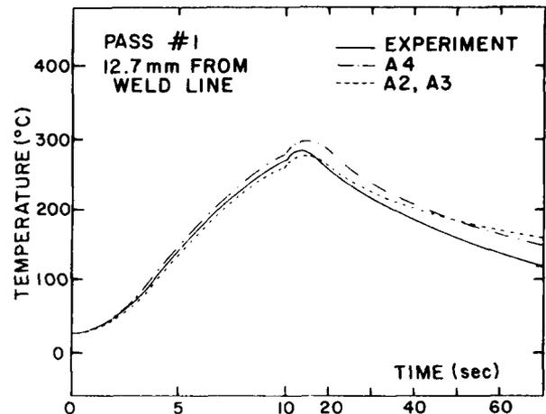
Fig. 6 Comparison of finite element results with experimental data (weld pass No. 1)
