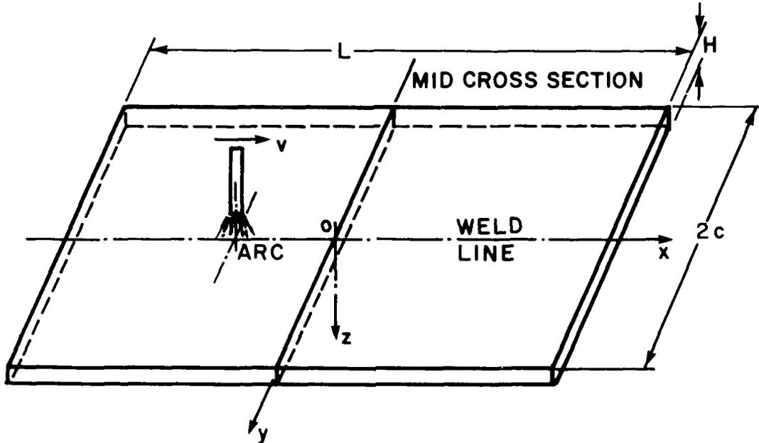
FIGURE 3.3 Weldment configuration (Butt welding of plates)
