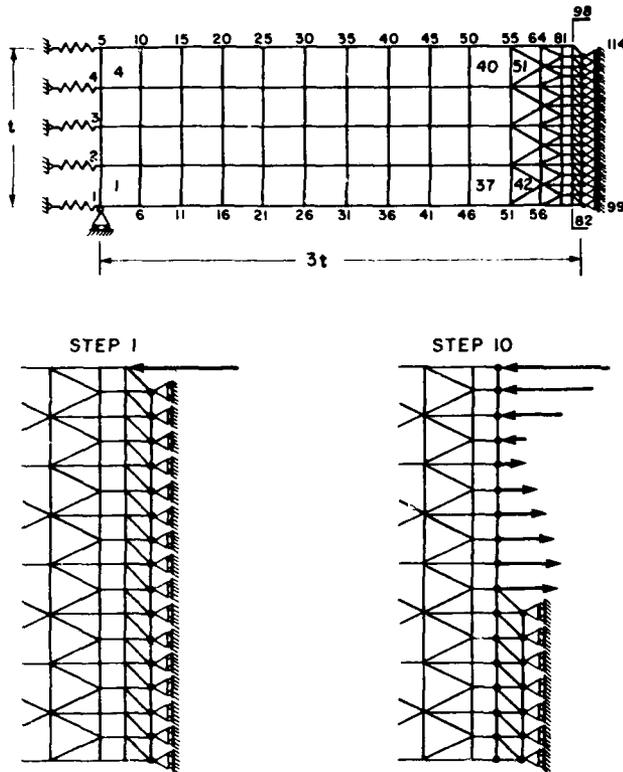
Fig. 19 Finite-element mesh used for the approximate calculation of the through-thickness residual stress distribution
