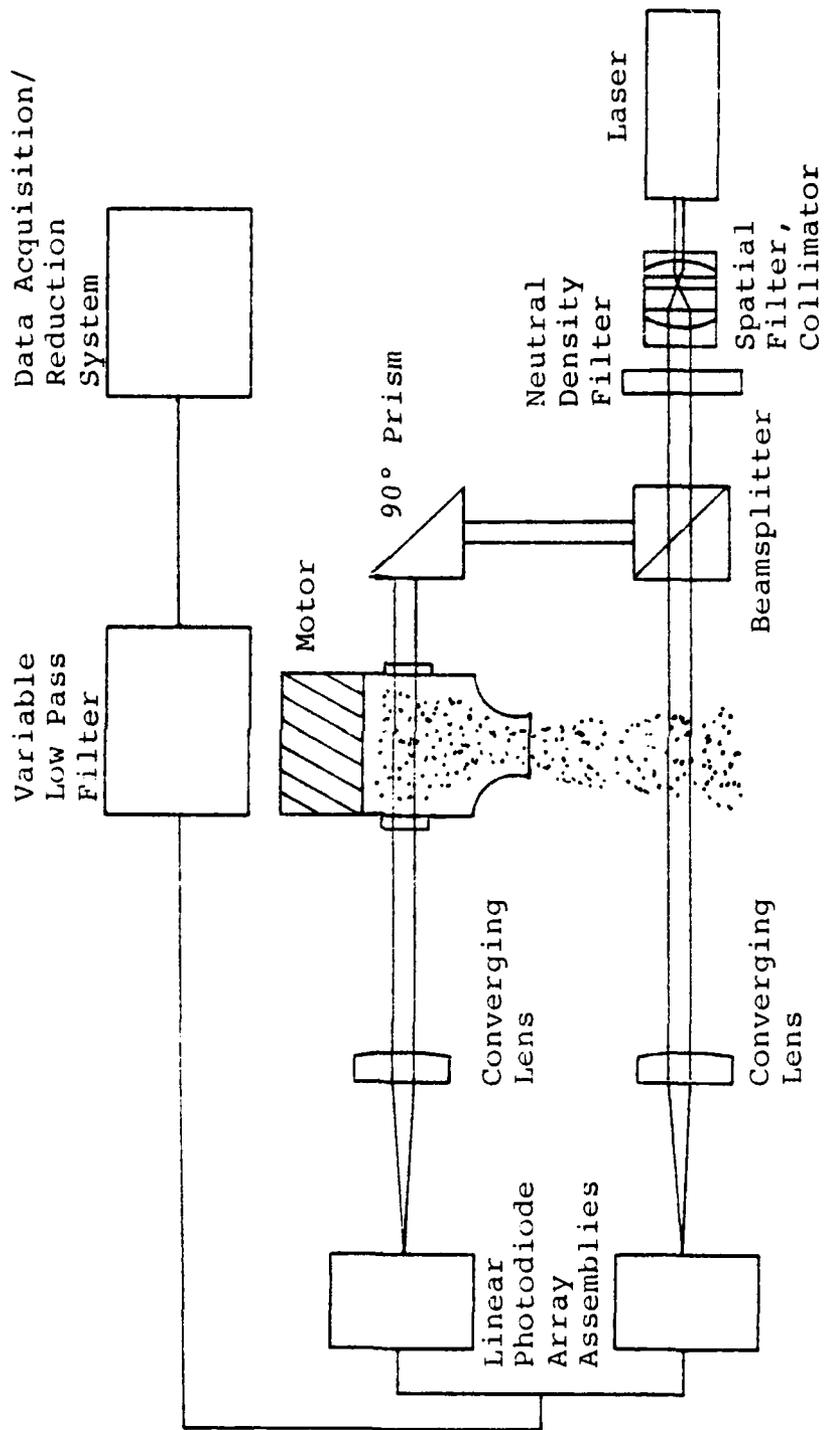
Figure 1: Schematic Diagram of Diffractively Scattered Light Apparatus
