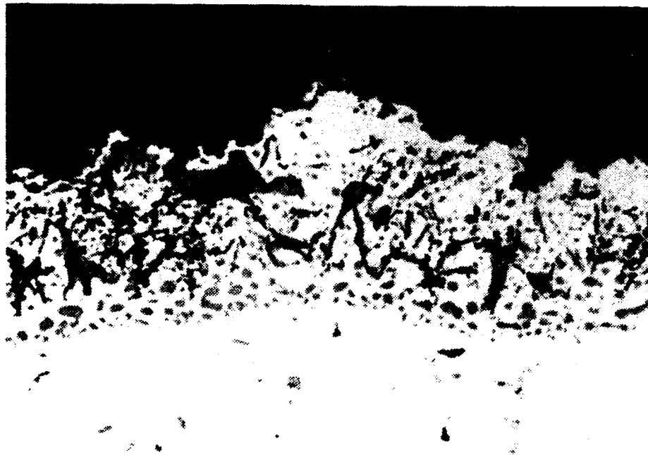
Figure 10. Type 1 Hot Corrosion in IN 738 Substrate after Outward Aluminide Coating was Consumed (500 Hours at 900°C), 650X, unetched
