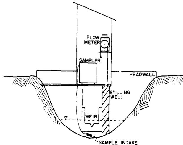
Figure 17. Interceptor ditch monitoring and sampling station.
