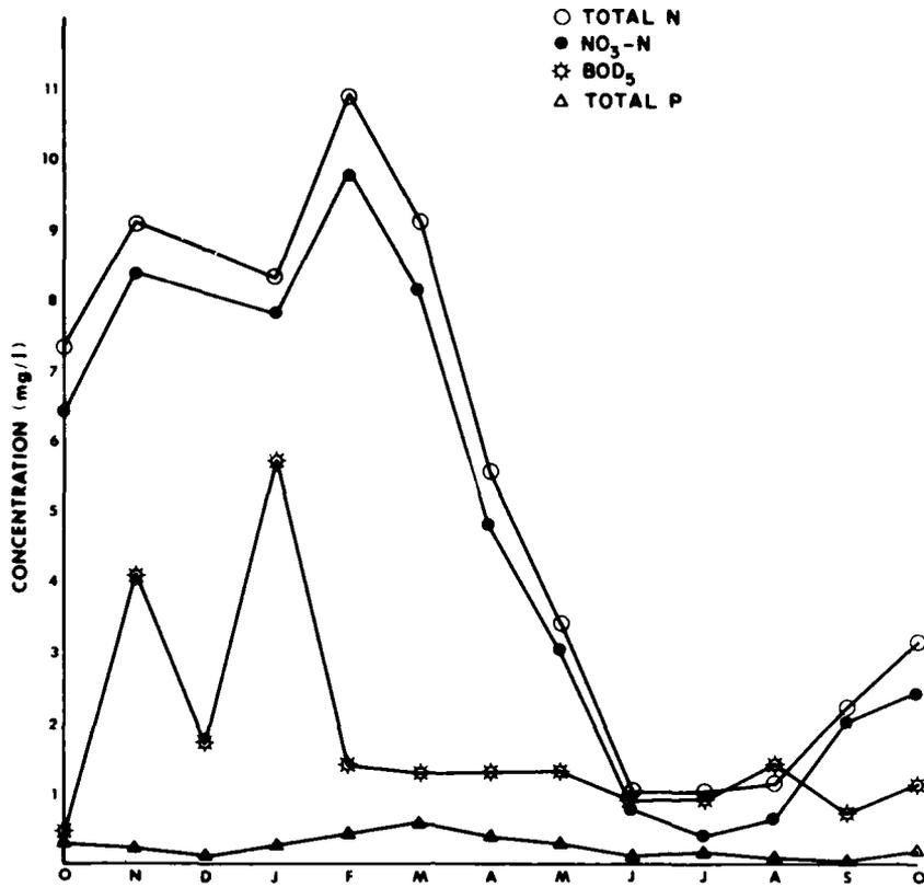
Figure 21. Monthly average concentration of total N, NO<sub>3</sub>-N, BOD<sub>5</sub> and total P in interceptor ditch flow.
