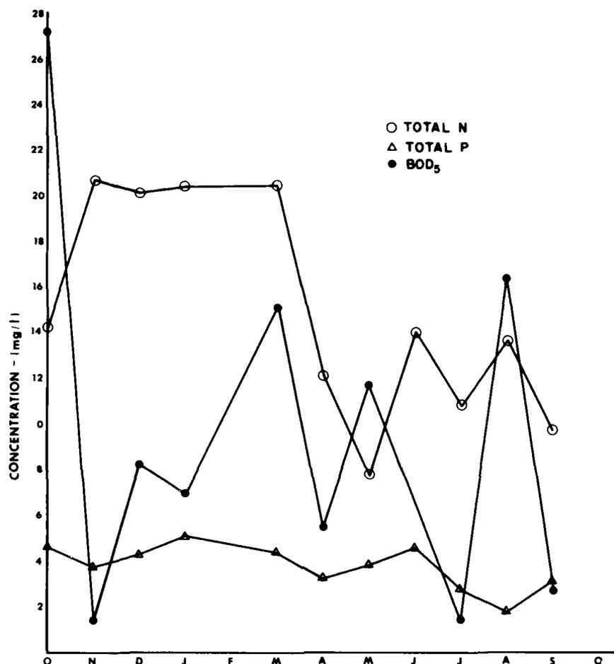
Figure 20. Monthly average concentration of total N, total P and BOD<sub>5</sub> in applied effluent.
