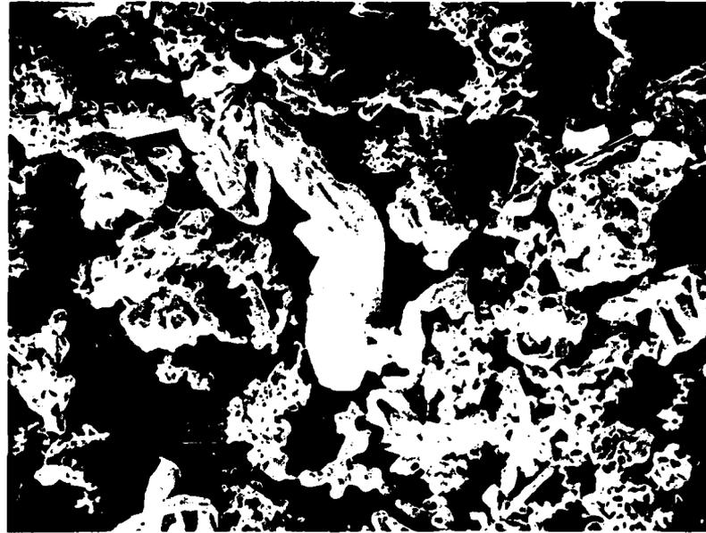
Figure 2. RMI Ti-020, -100 Mesh CP Ti Powder, SEM.
