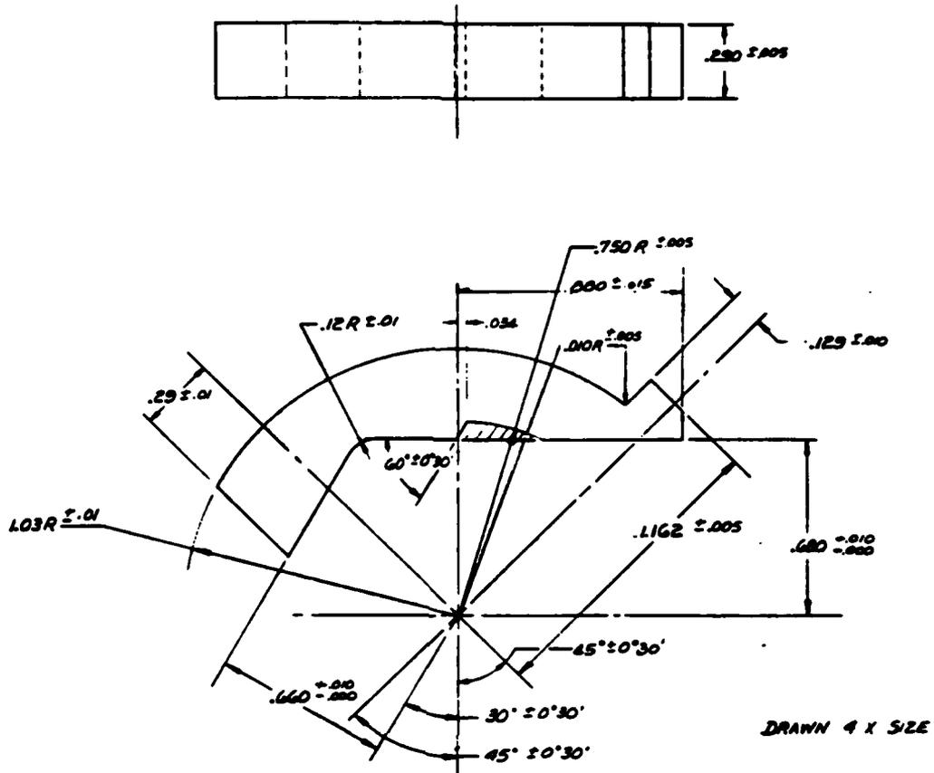
Figure 11. Actuator Housing Machining Preform, 408B
