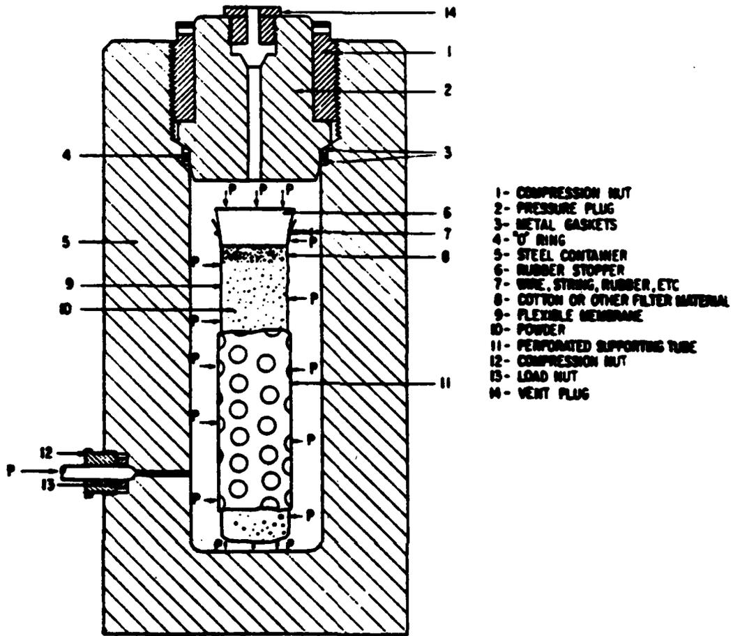
Sketch of a typical hydro-pressing assembly. The pressure is supplied by an auxiliary pumping unit.
