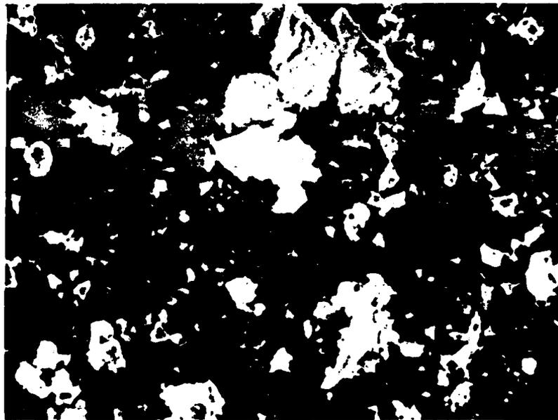
**Figure 3. Ball-milled Al-V, SEM.**
