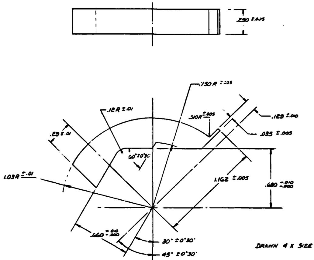
Figure 10. Actuator Housing Machining Preform, 408A.
