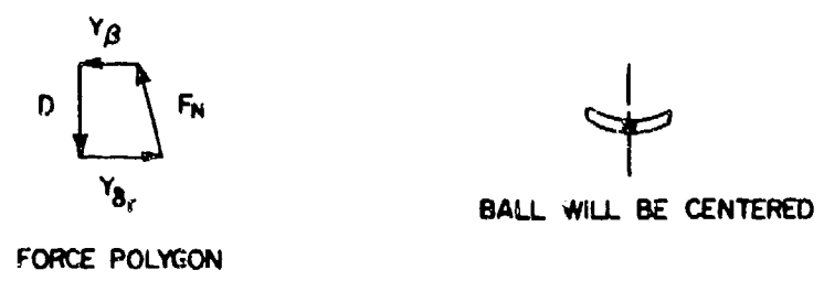
FIGURE 103 EQUILIBRIUM ASYMMETRIC POWER CONDITION WITH ZERO BANK ANGLE
