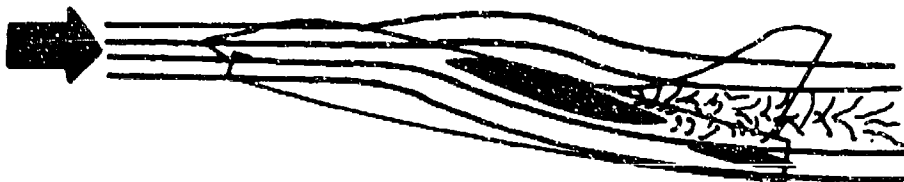
FIGURE 12 TYPICAL FLOW PATTERN AROUND THE VERTICAL TAIL AT HIGH ANGLE OF ATTACK
