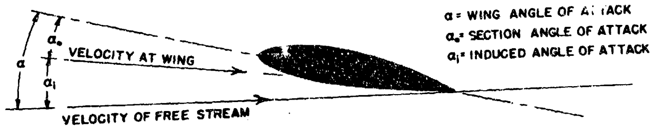
FIGURE 4 DOWNWASH INFLUENCE ON SECTION ANGLE OF ATTACK
