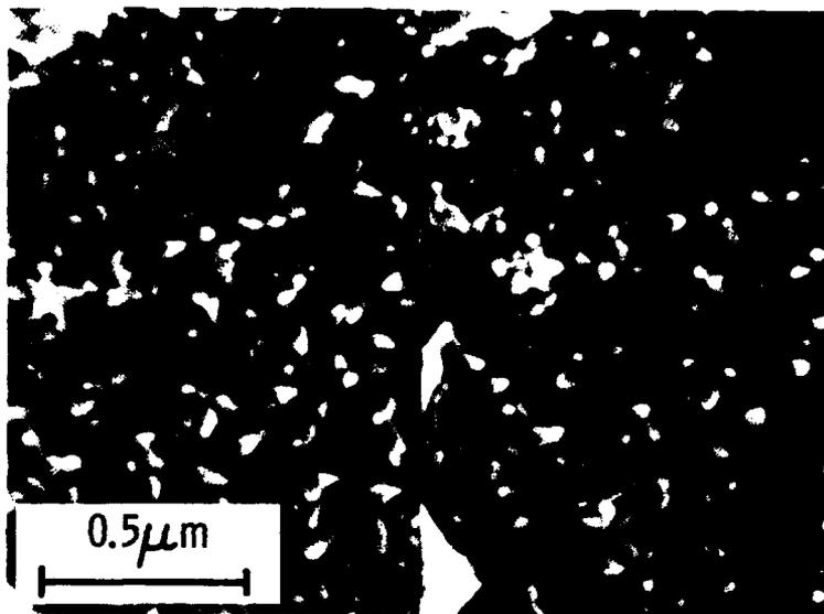
Figure 14. "Clean" Ti-6-4 surface after immersion in water at 95°C for 24 hours. Note the resemblance between this morphology and that of Fig. 13e.
