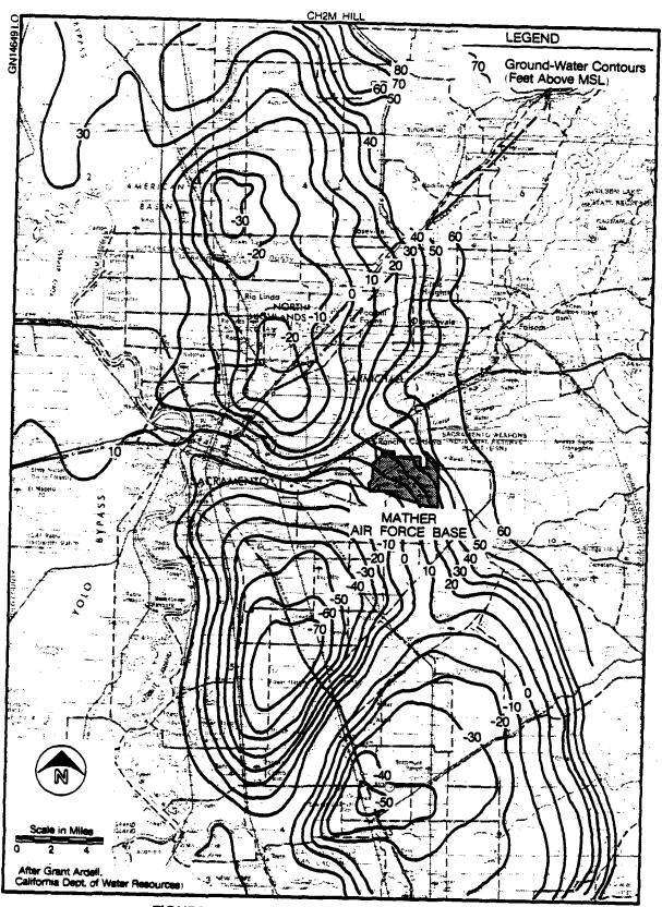
FIGURE 19. Ground-water contours-Spring 1980.
