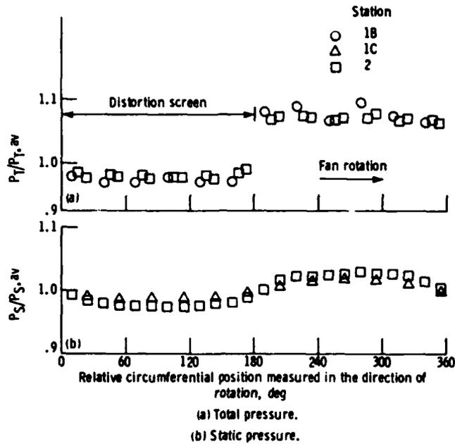
Figure 17. - Circumferential variation of total and static pressure with axial distance along inlet duct. Distortion screen is 180° and 49.4-percent blockage. Corrected fan speed, 90 percent; 0.5 RNI.
