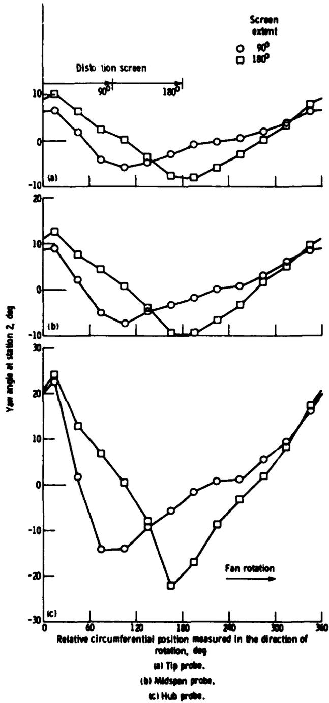
Figure 12. - Effect of screen extent on yaw-angle variation at station 2 for a 49.4-percent blockage screen. Corrected fan speed of 90 percent and 0.5 R/W.
