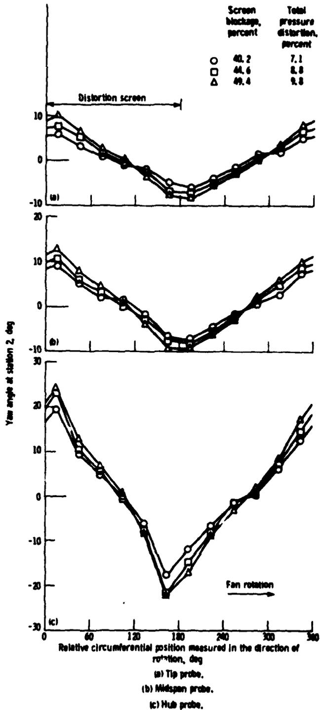
Figure 11. - Comparison of three screen blockages of 180° on yaw-angle variation at station 2. Corrected fan speed of 90 percent and 0.5 RNI.
