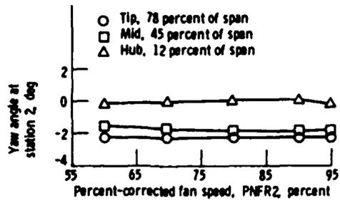
Figure 6. - Flow angle at station 2 (engine inlet) versus percent-corrected fan speed with no pressure distortion (clean inlet), 0.5 RNI.
