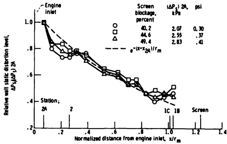
Figure 15. - Comparison of three screen blockages of 180° on static pressure distortion along inlet-duct wall. Corrected fan speed, 90 percent; 0.5 RNI.
