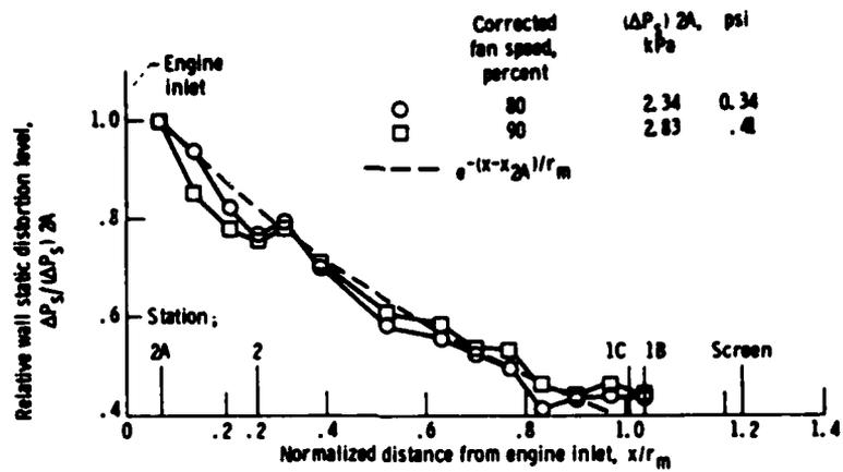
Figure 13. - Effect of percent-corrected fan speed on static pressure along inlet-duct wall for  $180^\circ$ , 49.4-percent blockage screen; 0.5 RNI.
