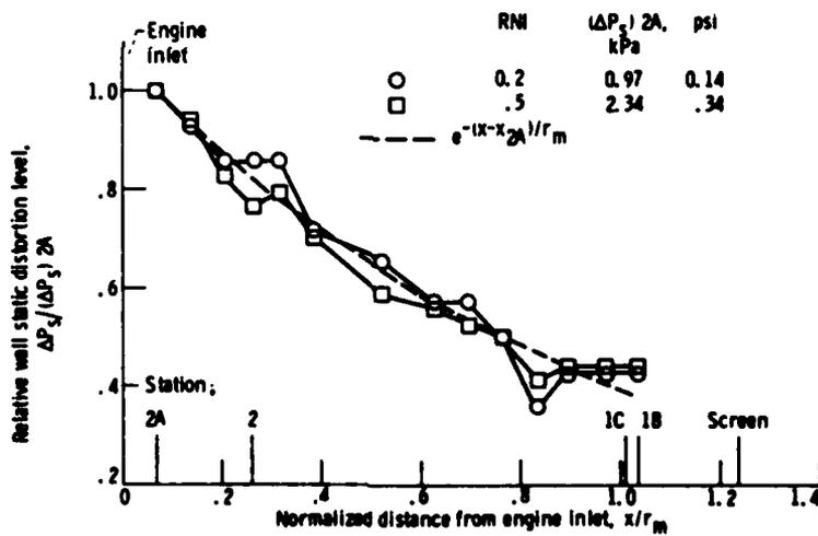
Figure 14. - Effect of RNI on static-pressure distortion along inlet-duct wall for  $180^\circ$ , 49.4-percent blockage screen; corrected fan speed, 80 percent.
