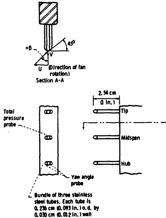
Figure 5. - Sketch of station 2 yaw-angle measurement rate.
