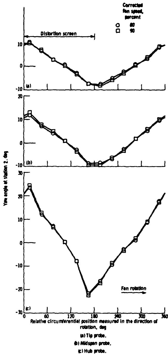
Figure 9. - Effect of corrected fan speed in percent on yaw-angle variation at station 2 for 180°, 49.4-percent blockage (9.8 percent total-pressure distortion) with 0.5 RNI.
