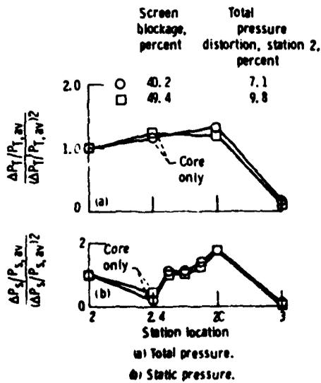
Figure 29. - Effect of screen blockage on pressure-distortion at station 2 variation. Corrected fan speed, 90 percent; 0.5 RNI.
