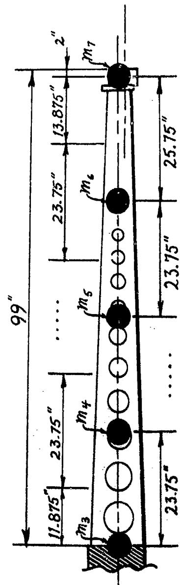
Figure 29 - Support Tube Simulation
