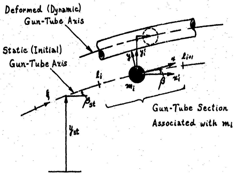
Figure 33 - Coordinate Relations for "Bourdon" and Projectile Induced Loads
