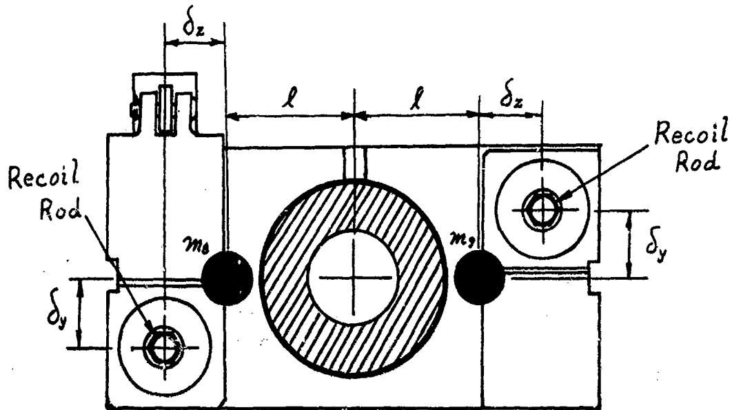
Figure 32 - Recoil Rod Offset
