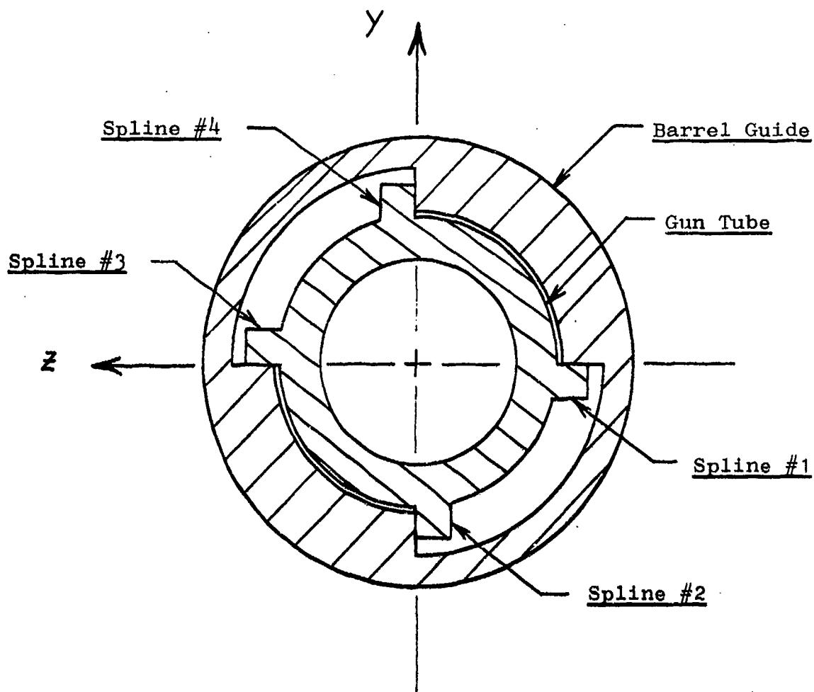
Figure 15 - Barrel Guide/Gun Tube Cross-Section
