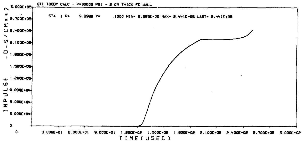
**Figure 5. Reflected Pressure and Impulse at 30,000 PSI**
