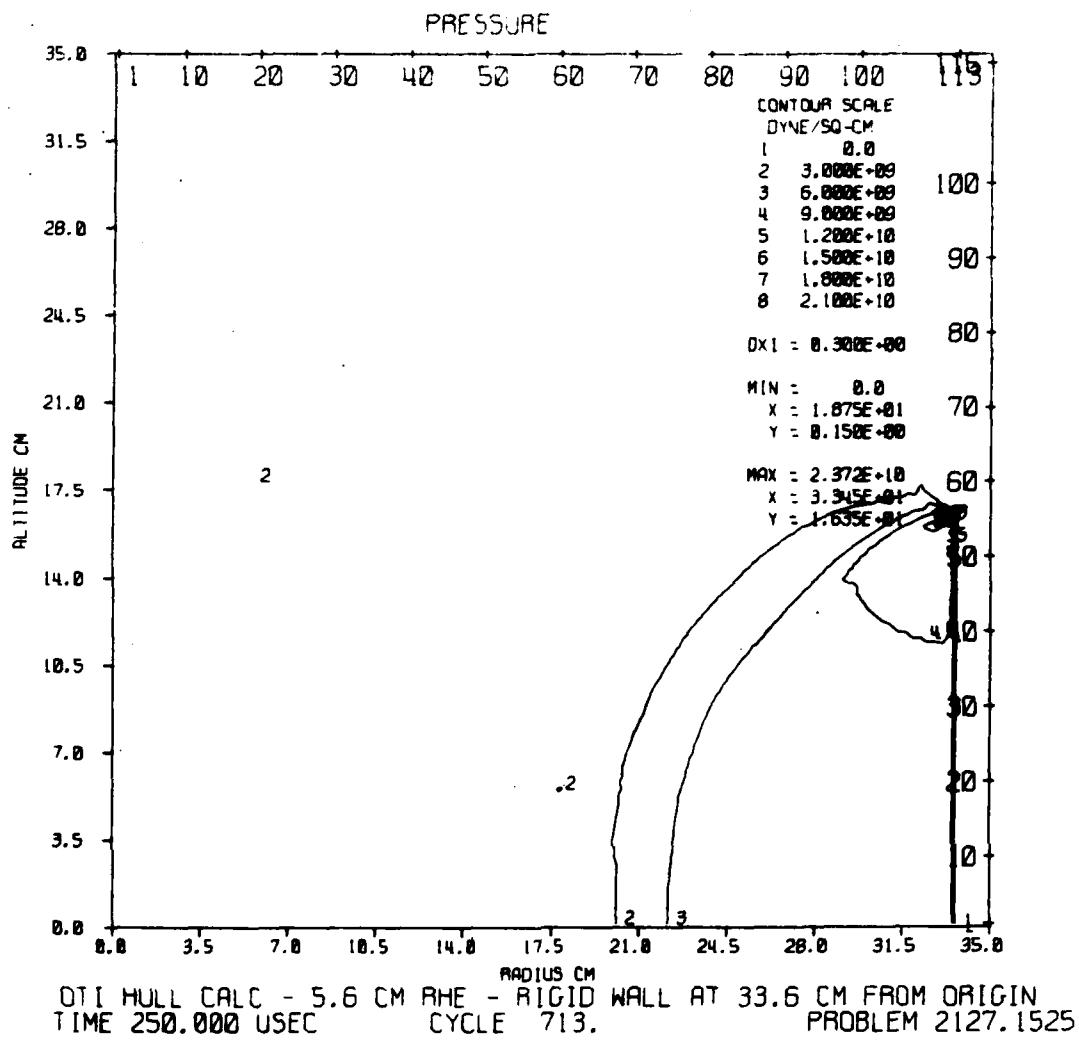
Figure 37. Pressure Contours at 250 Microseconds
