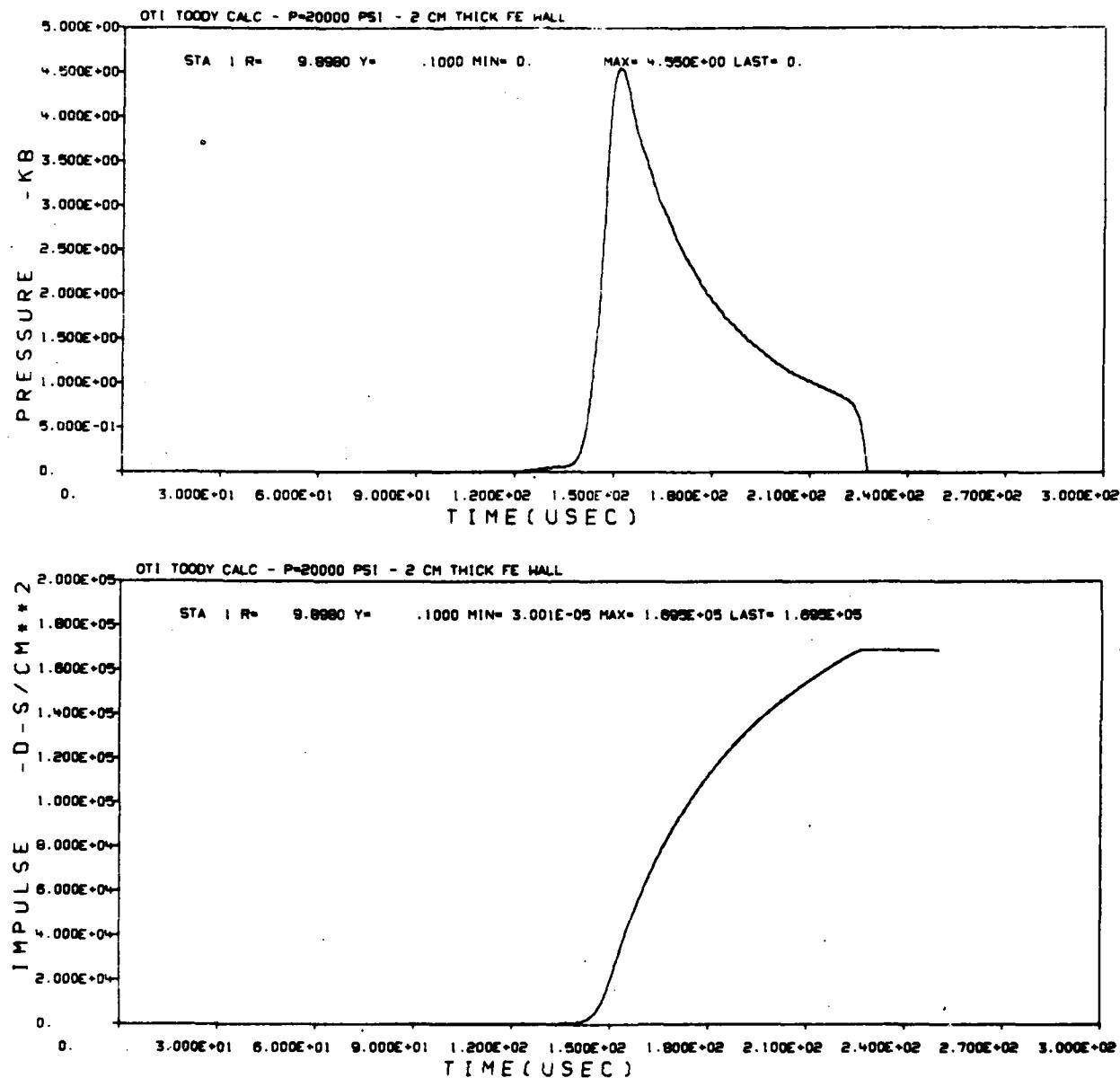
Figure 4. Reflected Pressure and Impulse at 20,000 PSI
