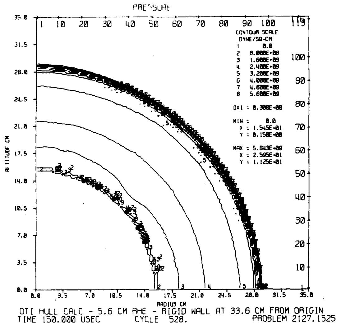
Figure 28. Pressure Contours at 150 Microseconds
