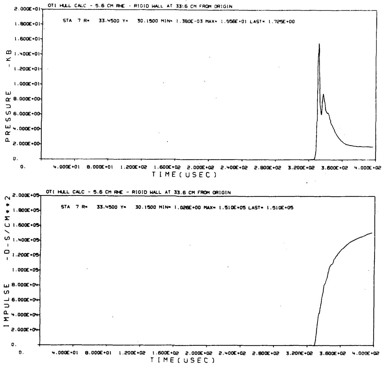
Figure 54. Station 7 Pressure/Impulse at Rigid Wall
