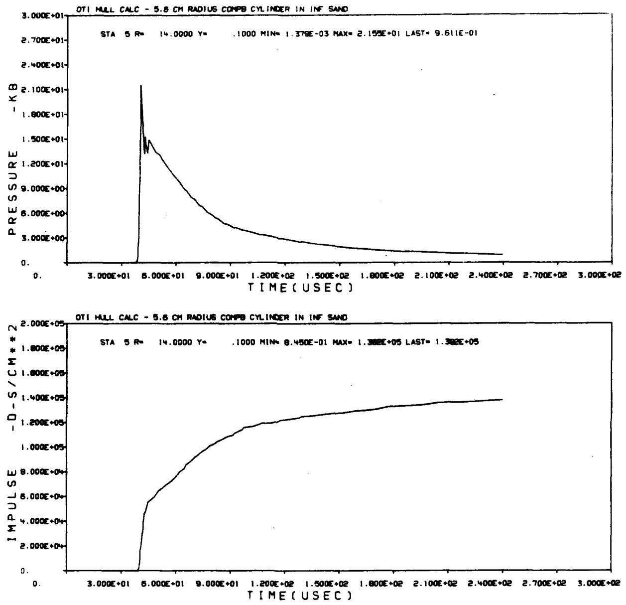
Figure 13. Station 5 Free-Field Pressure and Impulse
