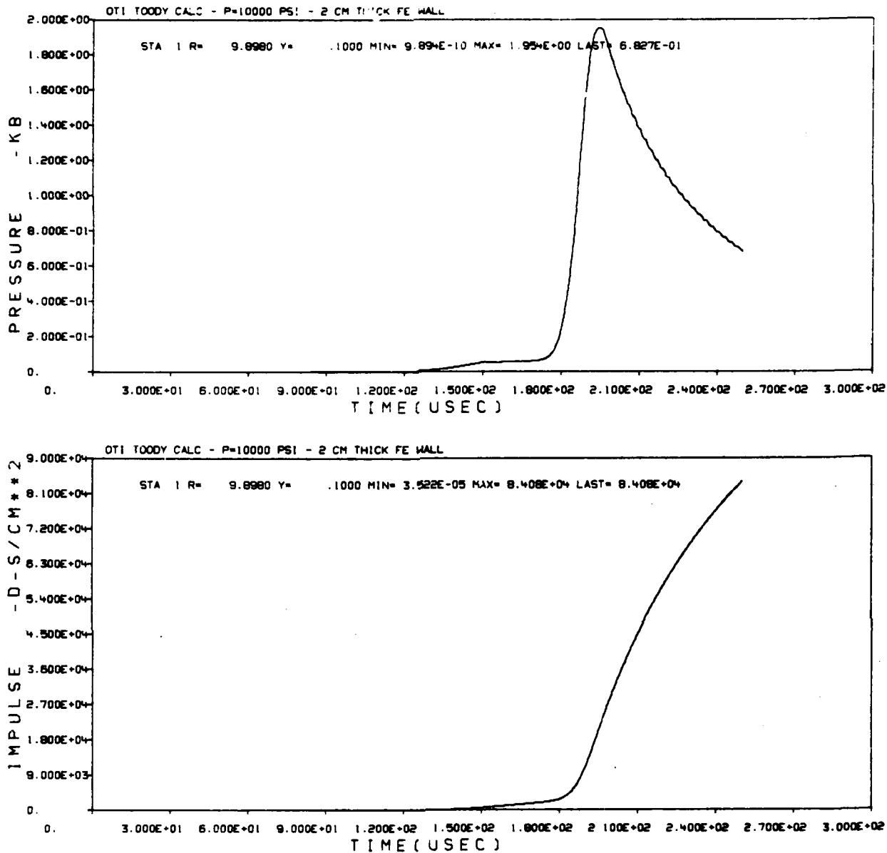
Figure 3. Reflected Pressure and Impulse at 10,000 PSI
