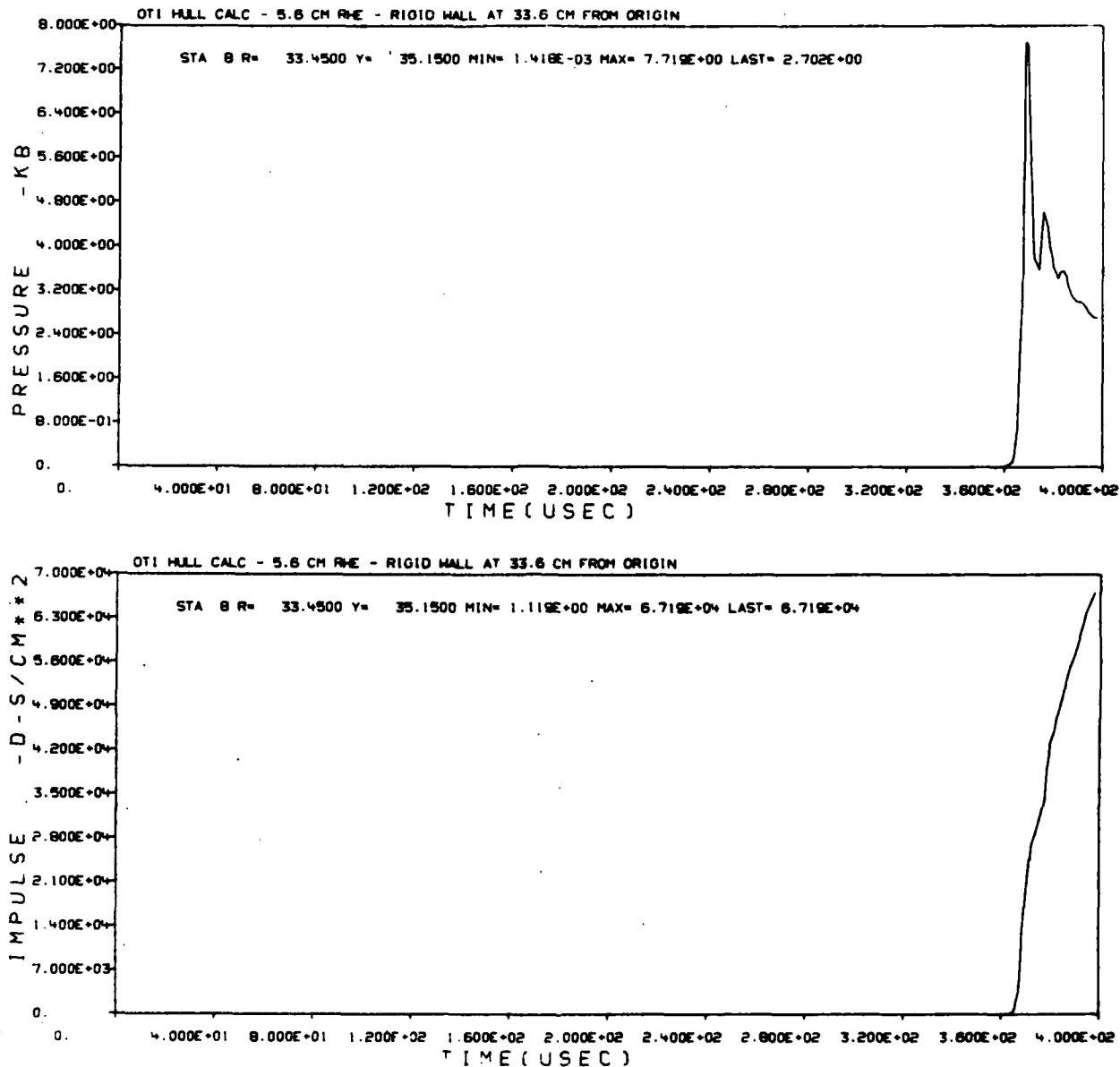
Figure 55. Station 8 Pressure/Impulse at Rigid Wall
