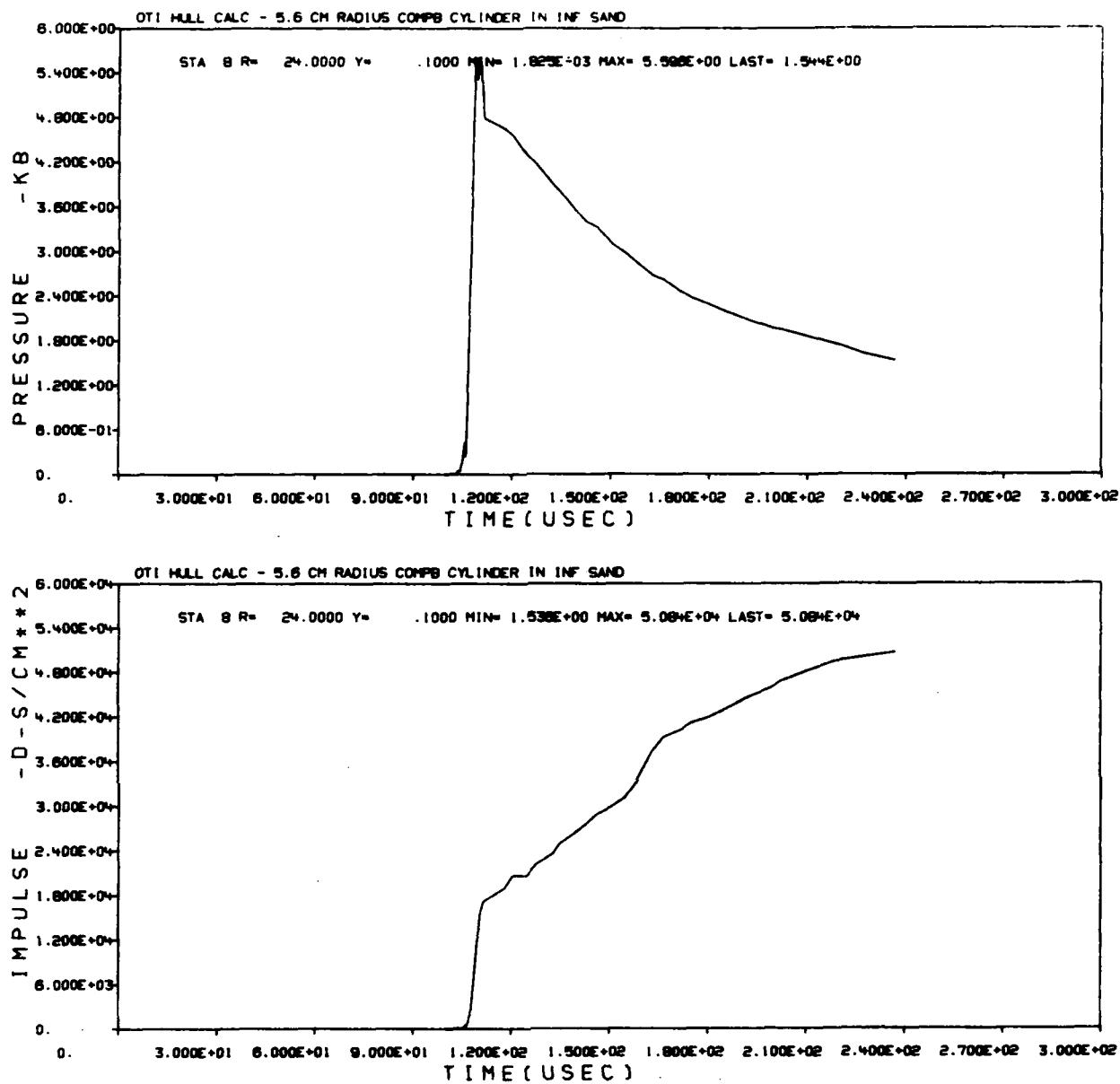
Figure 16. Station 8 Free-Field Pressure and Impulse
