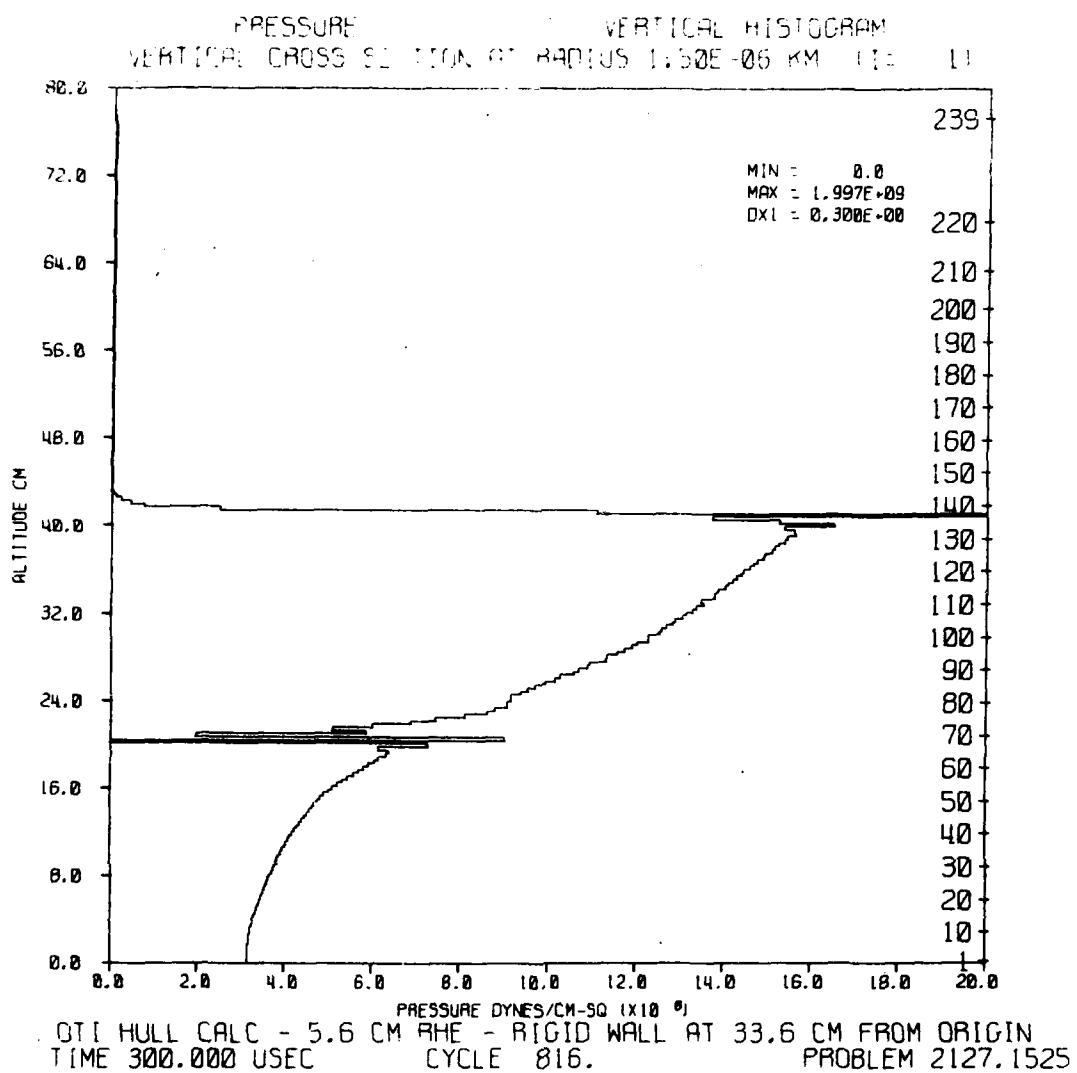
**Figure 41. Pressure Histogram at 300 Microseconds**
