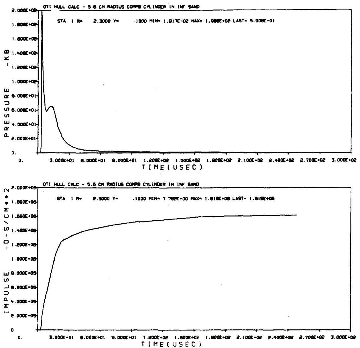
Figure 9. Station 1 Free-Field Pressure and Impulse
