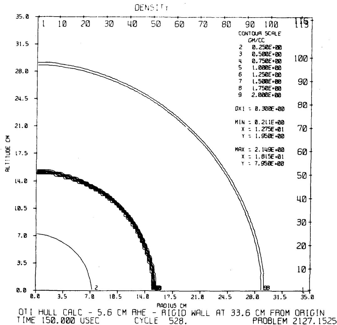
Figure 27. Density Contours at 150 Microseconds
