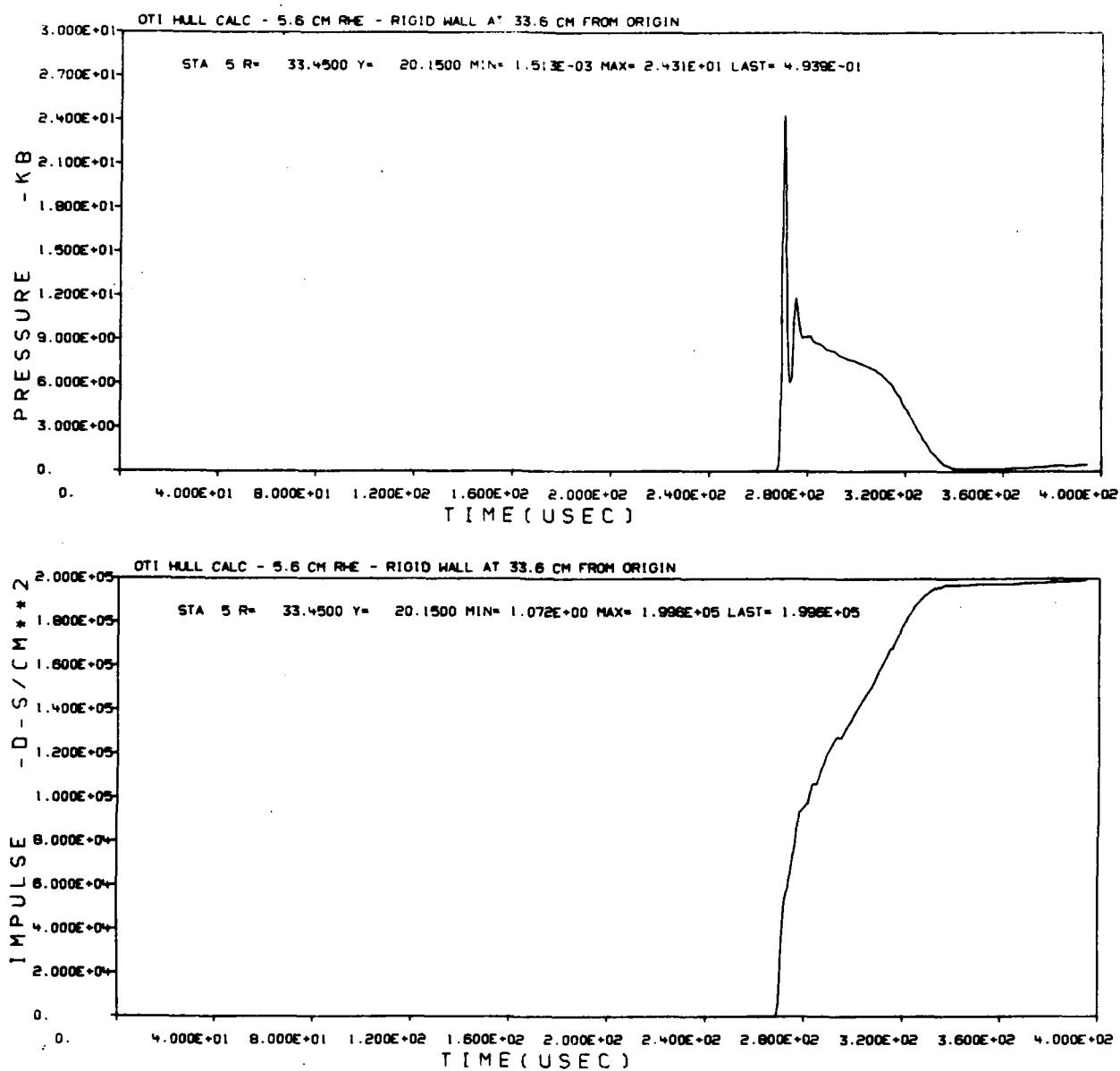
Figure 52. Station 5 Pressure/Impulse at Rigid Wall
