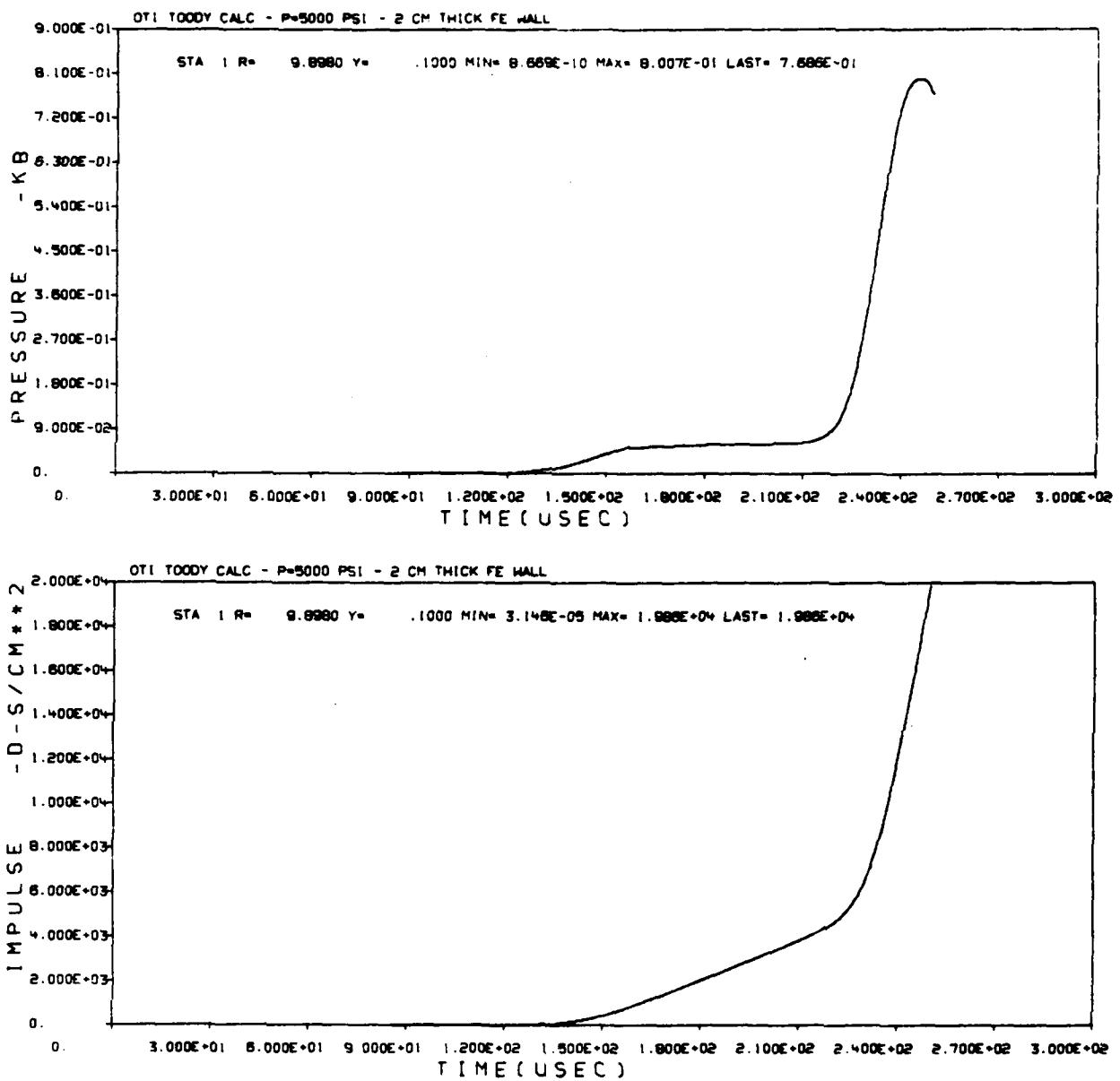
Figure 2. Reflected Pressure and Impulse at 5000 PSI
