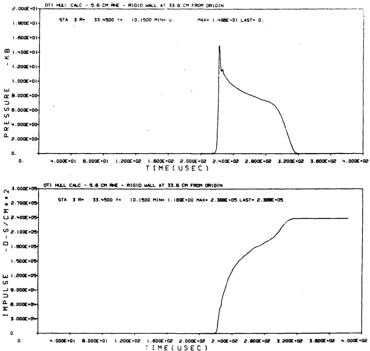
Figure 50. Station 3 Pressure/Impulse at Rigid Wall
