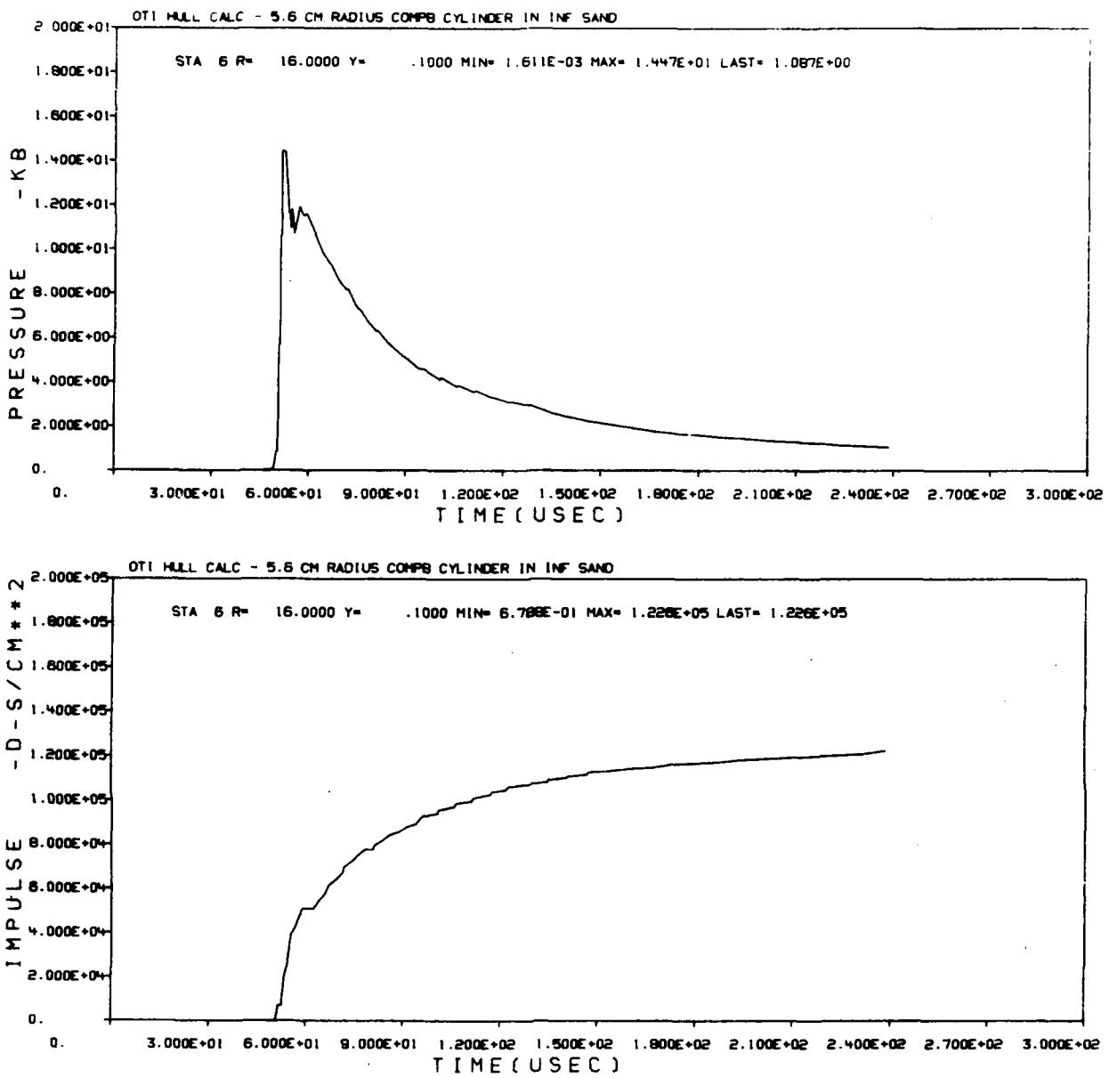
Figure 14. Station 6 Free-Field Pressure and Impulse
