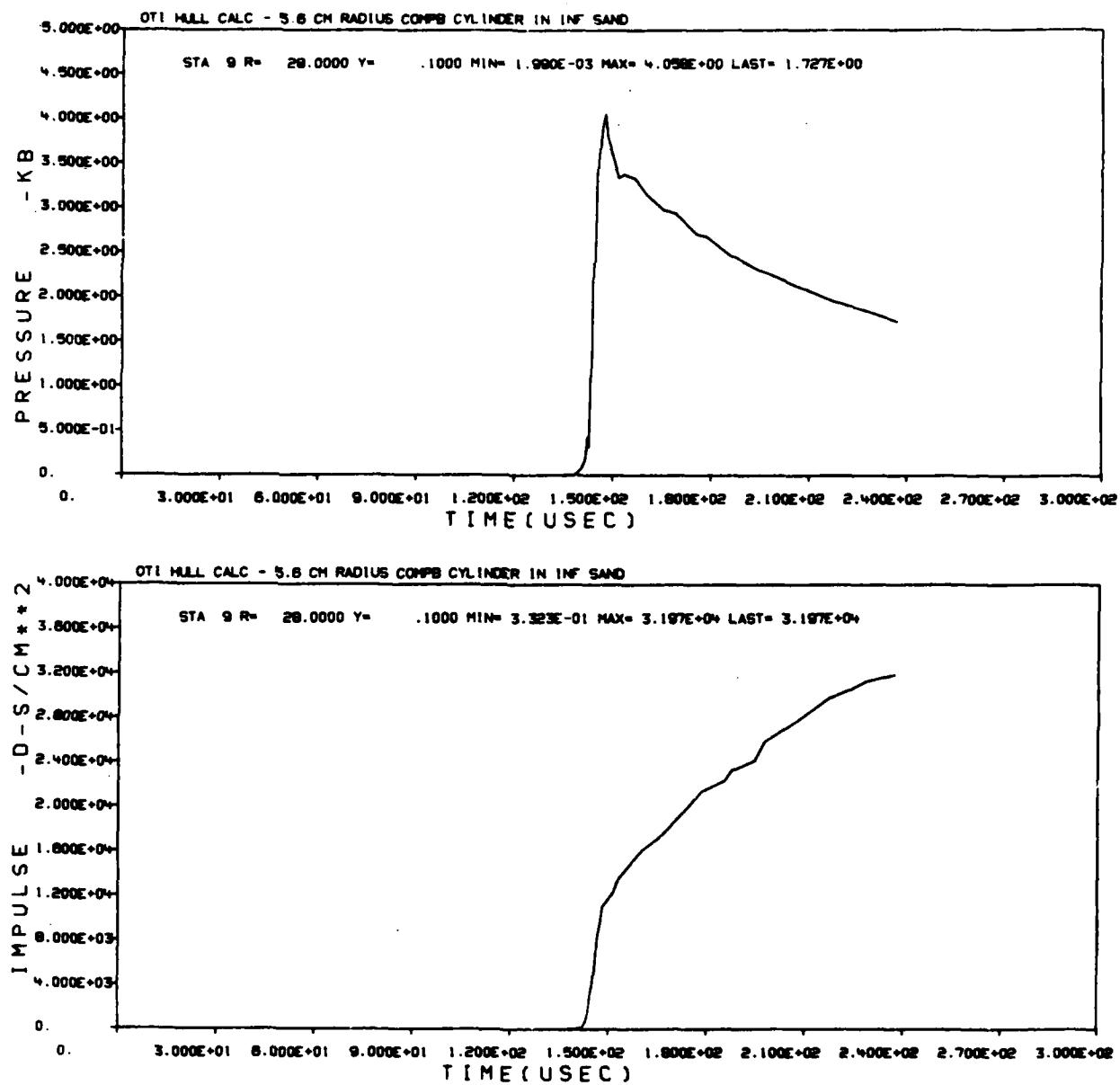
Figure 17. Station 9 Free-Field Pressure and Impulse
