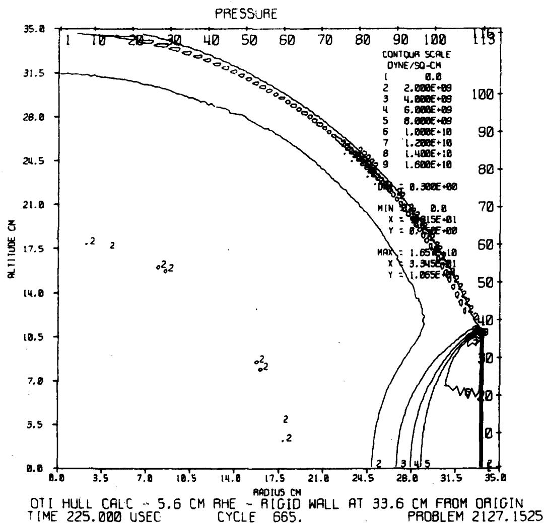
Figure 34. Pressure Contours at 225 Microseconds
