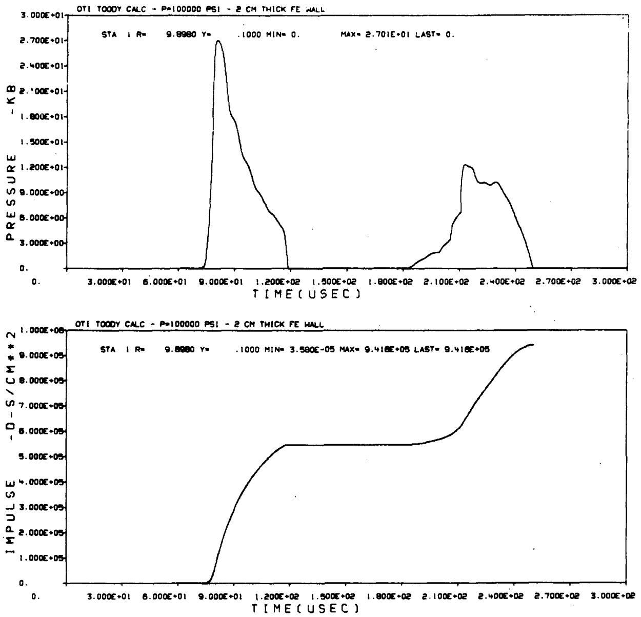
Figure 7. Reflected Pressure and Impulse at 100,000 PSI
