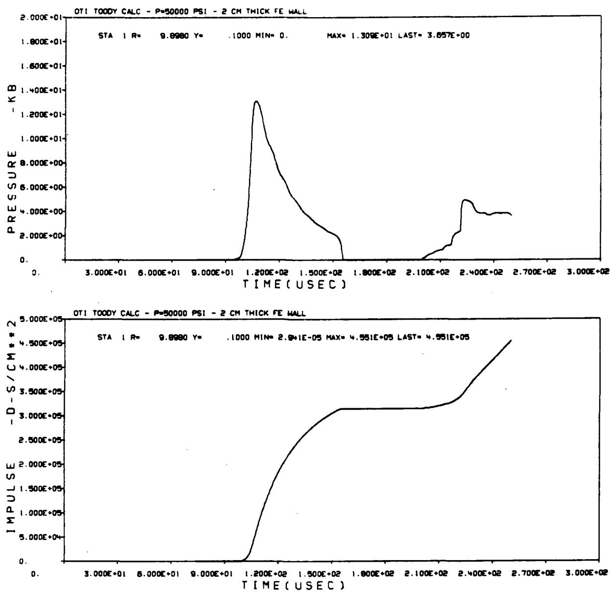
Figure 6. Reflected Pressure and Impulse at 50,000 PSI
