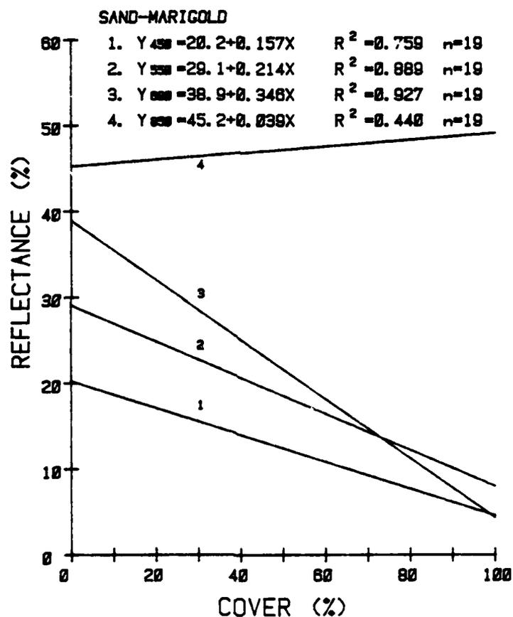
FIGURE 7. Regression Curves for Reflectance at 450, 550, 680 and 850 nm and Percent Cover of Sand-Marigold Targets.
