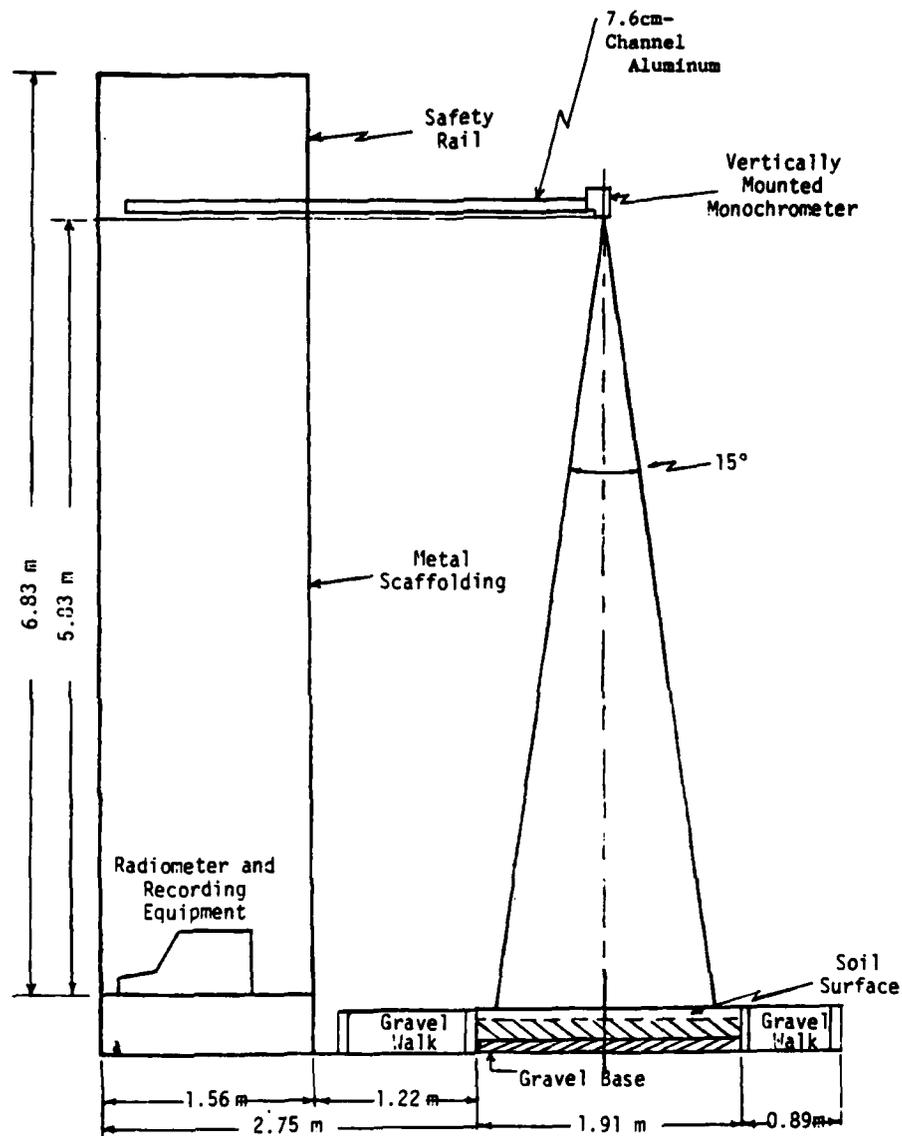
FIGURE 2. A Schematic Side View of the Monochrometer Position Over a Test Plot.
