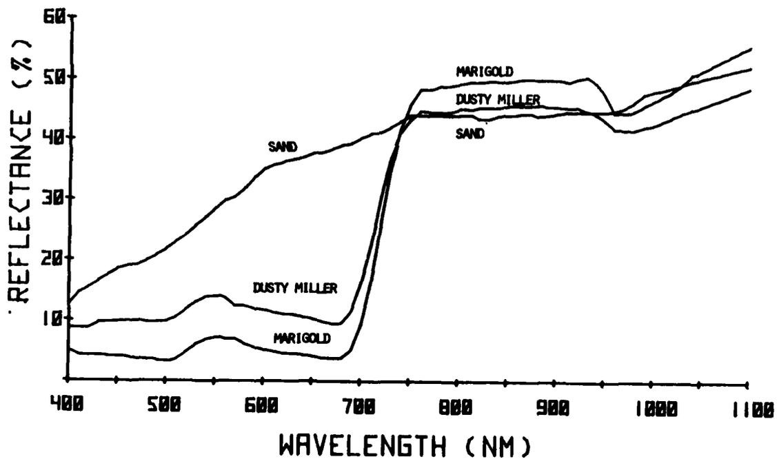
FIGURE 5. Measured Reflectance Curves for Sand Soil, Marigold and Dusty Miller.
