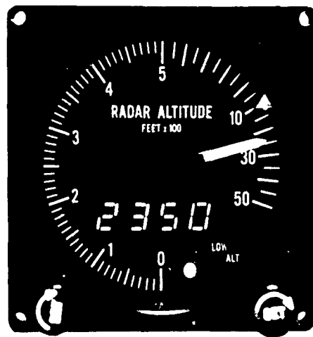
Fig.3.5.10 Photograph of an operating f-111 green led numeric readout low altitude radar altimeter
