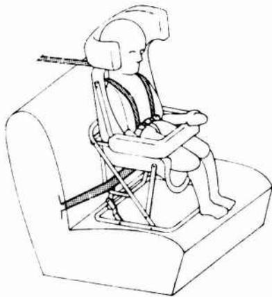
Figure 3 Test set up of a child in a harness type child restraint system.
