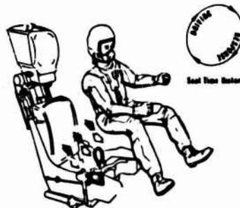
Figure 3. Rocket phase of ejection. Note the closed loop system where occupant response influences seat trajectory.
