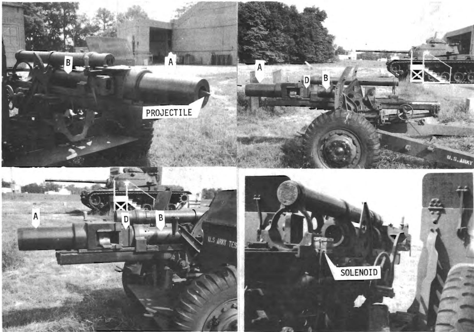
Figure 2. Modified M2A2 Tube Mounted in M101, Towed System.
