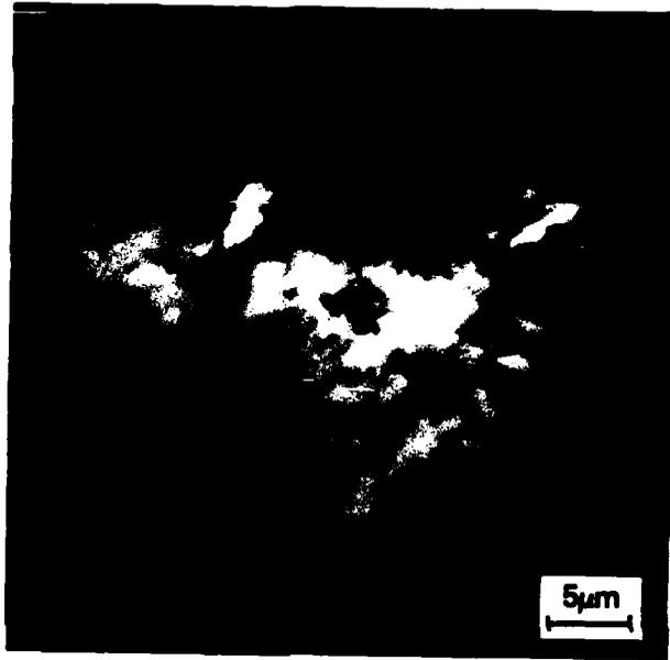
Figure 5. Oxide debris extruded from crack flank in MA-87 cycled in air,  $\Delta K \approx 10 \text{ MNm}^{-3/2}$ .
