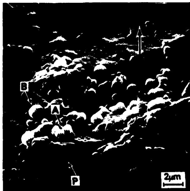
Figure 2. Spheroidal wear debris on fatigue fracture surface of MA-87, vacuum environment,  $\Delta K = 7 \text{ MNm}^{-3/2}$ . Platelet (P), separated spheroids (A), lapped spheroid (B). Large arrow shows direction of crack growth.
