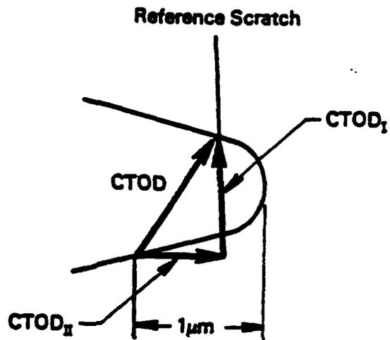
Figure 1. Schematic of crack tip opening parameters, showing displacement of a hypothetical reference mark 1 μm behind the crack tip.
