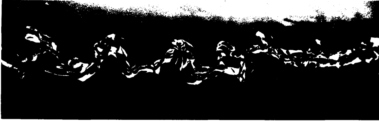
Figure 17. The helical phase becomes more exaggerated in a polymer jet, 192 diameters downstream.
