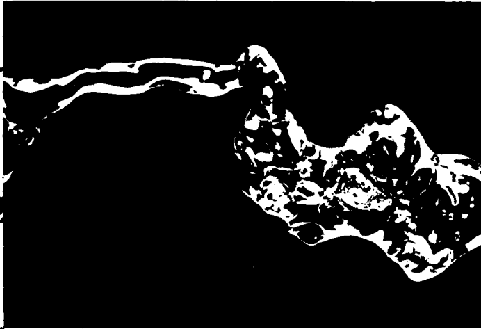
Figure 10. The jet has almost disintegrated due to its corkscrew-like motion.
