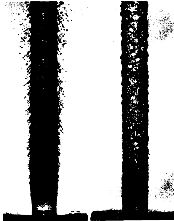
Figure 15. The polymer jet (below) is discharging at the same pressure and from the same nozzle as the water jet above. Transition to turbulence occurs inside the nozzle when polymers are used.
