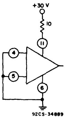
Fig. IV-3 - CA741 250°C bias-life-test circuit.
