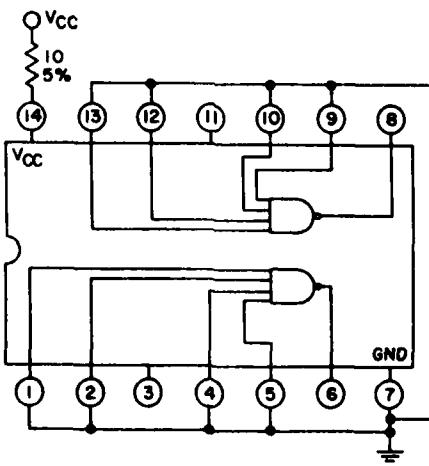
$V_{CC} = 5.375 \text{ V} \pm 0.125 \text{ V}$
