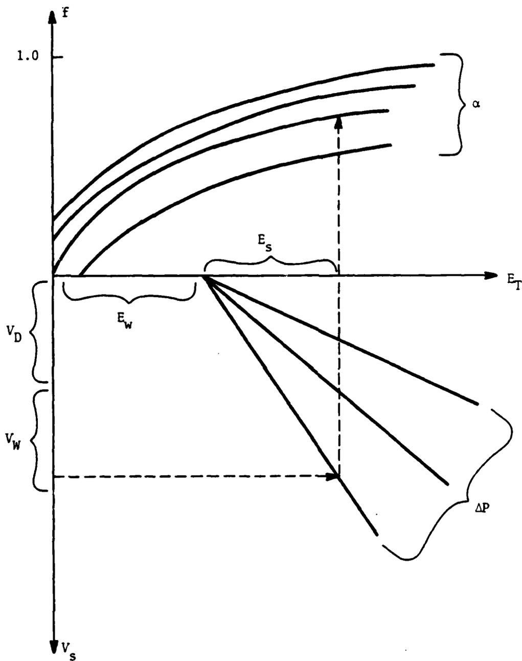
FIGURE B.1. RELATIONSHIPS AMONG PARAMETERS OF A VESSEL-MOUNTED SPRAY BOOM SYSTEM
