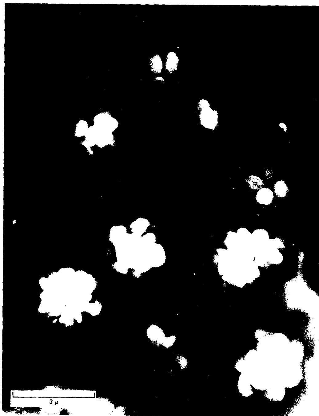
FIGURE 12 PHASE SEPARATION IN Mg-Si-O-N GLASS Light phase is SiO 2 -rich, matrix is magnesium-rich (Reference 36)
