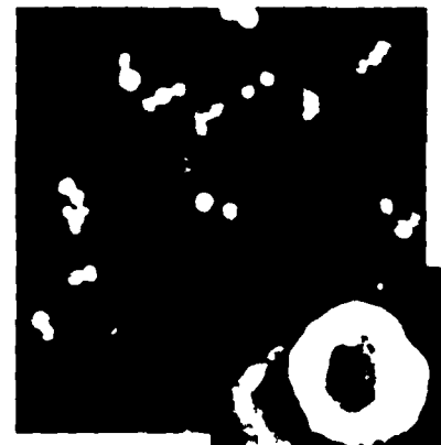
(e) Crystalline spheres, mag. 200\times , polarized light. (Inset shows SEM of one sphere, mag. 1000\times .)
