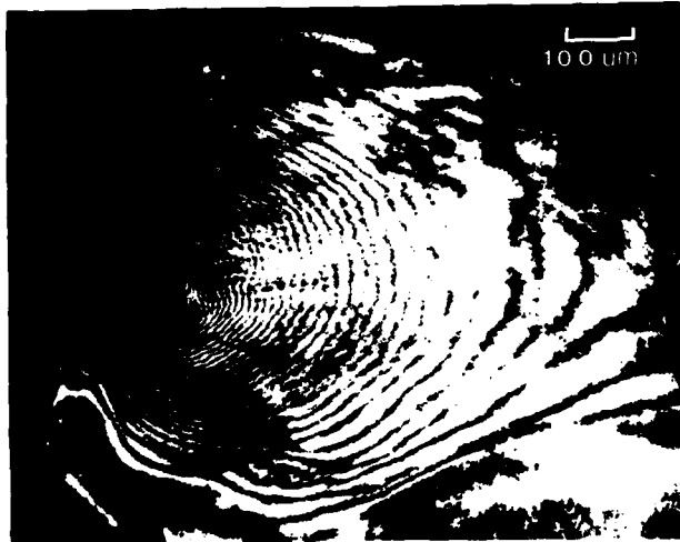
Fig. 4. (shot 4833) Nitrogen gas jet, 2000 psi; Laser jet irradiation, \lambda = 1.053 \mu\text{m} , 46.5 Joules in 85 psec. Laser holographic probe, \lambda = .2633 \mu\text{m} ; duration=60 psec; occurring 290 psec after peak of irradiating pulse.
