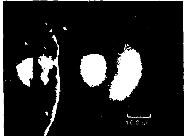
Fig. 5. Composite image of 2\omega and 3/2\omega harmonics of 1.05 \mu\text{m} laser light emitted by a hydrogen jet target.
