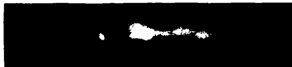
Fig. 1. Pinhole photograph of 7 Å plasma x-ray source - three shot overlay
