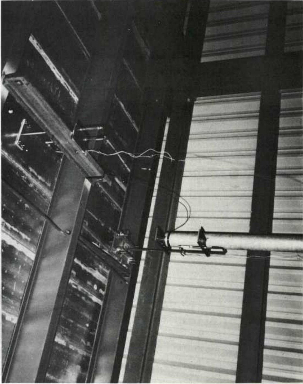
Figure 3. Typical deflection gage mount
