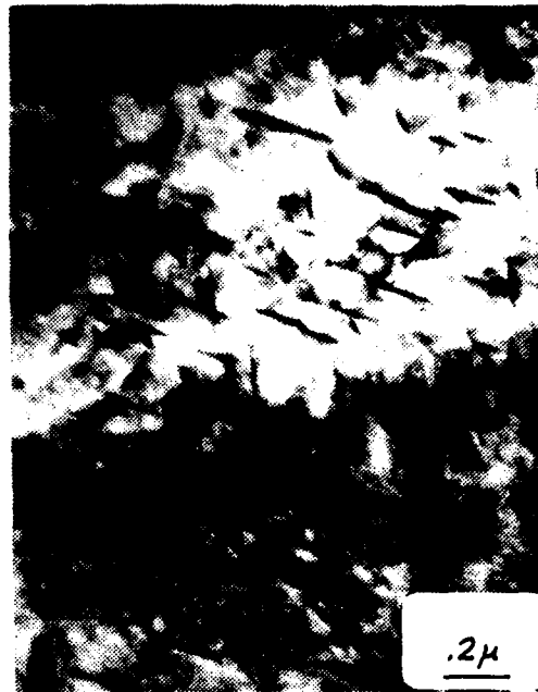
MICROSTRUCTURE AT 2.5mm. AWAY FROM THE FUSION LINE IN REGION 3 WITH THE PHOTO ON THE RIGHT AN ENLARGEMENT OF THE ROD-SHAPED WIDMANSTATTEN CARBIDES PRECIPITATED IN THE UPPER BAINITE ON THE LEFT
