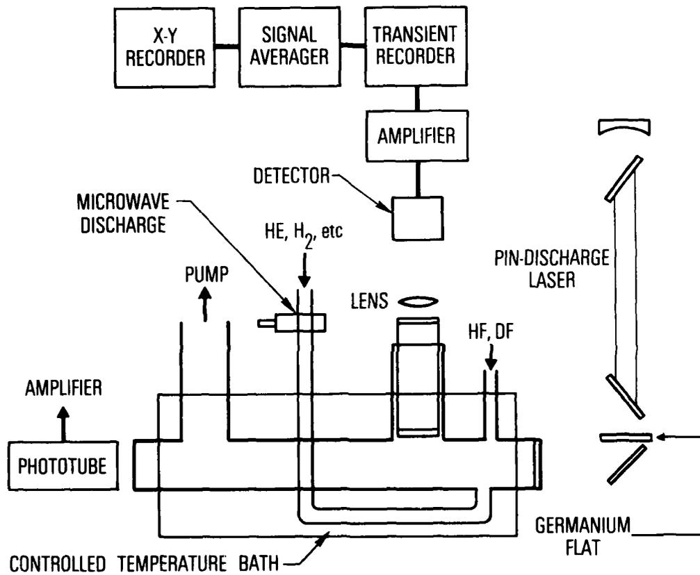
Fig. 1. Schematic of Apparatus
