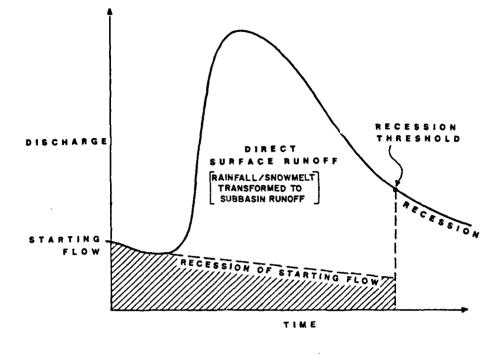
FIGURE 3 HEC-1 SUBBASIN RUNOFF SIMULATION
