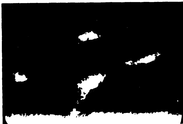
Fig. 4.10. A hologram of cavitation inception on the one-half inch blunt body. u_{\infty} = 21.1 ft/sec, Re_D = 8.24 \times 10^4 , \sigma = 1.41 .
