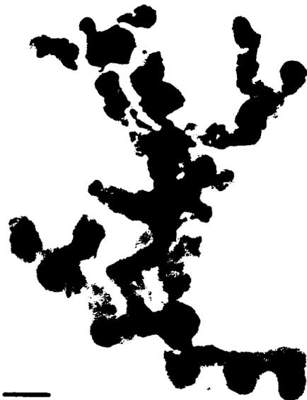
Figure 16. TEM photomicrograph of Si powders. Lot 634S. (Bar 500 Å)
