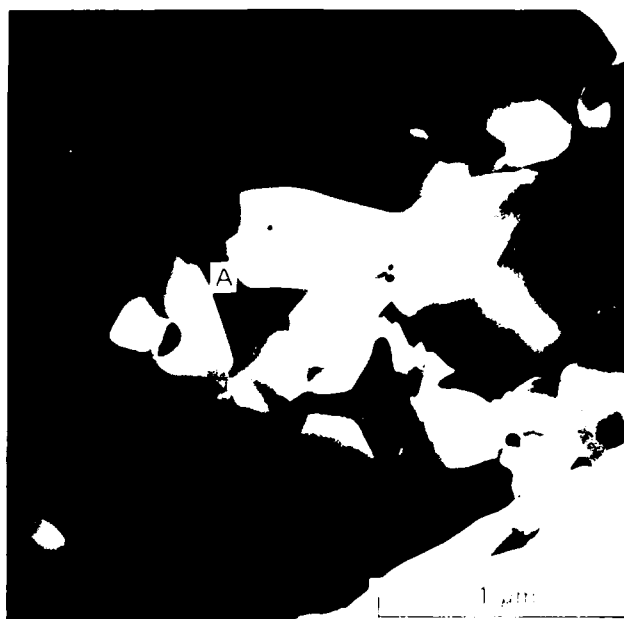
FIGURE 8 AMORPHOUS POCKET (A) IN \text{Si}_3\text{N}_4 ABOUT 0.25 mm AWAY FROM THE ORIGINAL GLASSY JOINT
