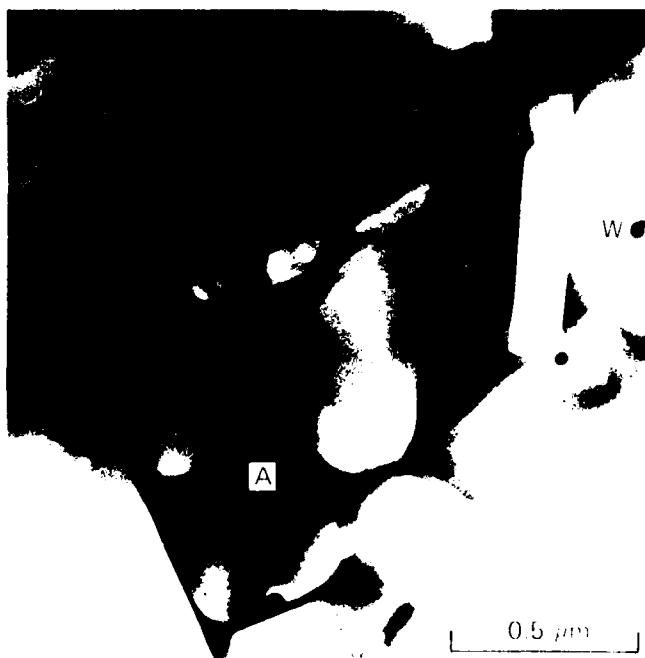
FIGURE 8 AMORPHOUS POCKET (A) IN \text{Si}_3\text{N}_4 ABOUT 0.25 mm AWAY FROM THE ORIGINAL GLASSY JOINT
